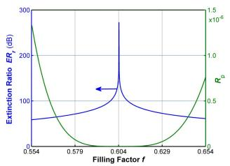
Fig. 2. (Color online) Intensity reflectance  $R_p$  and extinction ratio ER<sub>r</sub> (dB) of prism–PCL interface are plotted as functions of grating filling factor f. These calculations are for ZnTe 1-D PCL embedded in ZnS prism, with grating period  $\Lambda=1\mu m$ , wavelength  $\lambda=10.6\,\mu m$ , and 45° angle of incidence.
