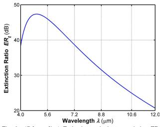
Fig. 8. (Color online) Extinction ratio in transmission  $\text{ER}_t$ , Eq. (9), plotted as a function of wavelength  $\lambda$  under the same conditions described in Fig. 7.
