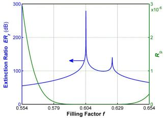
Fig. 5. (Color online) Intensity reflectance  $R_p$  and extinction ratio ER<sub>r</sub> of ZnTe 1-D PCL of thickness  $d = 10 \,\mu\text{m}$  embedded in ZnS cube plotted as functions of f for  $\lambda = 10.6 \,\mu\text{m}$ ,  $\Lambda = 1 \,\mu\text{m}$ , and  $\phi = 45^{\circ}$ . Interference effects in the PCL are accounted for.
