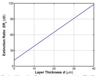
Fig. 9. (Color online) Extinction ratio in transmission ER<sub>t</sub> (dB), Eq. (9), plotted as a function of thickness  $d~(\mu m)$  for ZnTe 1-D PCL embedded in ZnS prism with f = 0.604 and at wavelength  $\lambda = 10.6\,\mu m$ .
