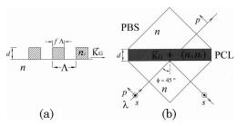
Fig. 1. (a) Cross section of 1-D PCL of thickness *d* that consists of rectangular grating of a coating material of refractive index  $n_c$ , period  $\Lambda$ , and filling factor *f*. The layer is deposited on an optically isotropic substrate (prism) of refractive index *n*. (b) Cube PBS using an embedded PCL with grating vector  $\vec{K}_G$  normal to the plane of incidence. *p* and *s* denote the linear polarizations parallel and perpendicular to the plane of incidence, respectively.
