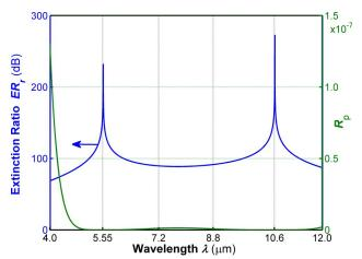
Fig. 4. (Color online) Intensity reflectance  $R_p$  and extinction ratio ER<sub>r</sub> plotted versus wavelength  $\lambda$ ,  $4 \le \lambda \le 12 \,\mu$ m, for a PBS that uses ZnTe 1-D PCL embedded in ZnS prism with grating period  $\Lambda = 1 \,\lambda$ m and filling factor f = 0.604. Dispersion of prism and coating materials is accounted for.
