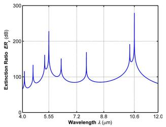
Fig. 7. (Color online) Extinction ratio in reflection ER<sub>r</sub> of ZnTe 1-D PCL of thickness  $d = 10 \,\mu\text{m}$ , f = 0.604, embedded in ZnS cube, shown as a function of wavelength  $\lambda$ . ER<sub>r</sub> has Fabry-Perot-type multiple peaks at wavelengths at which destructive interference for the *p* polarization occurs.
