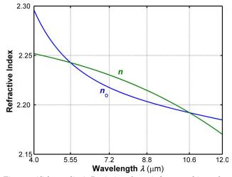
Fig. 3. (Color online) Deviation from index matching of *p*polarized light (i.e.,  $n_o = n$ ) as the wavelength  $\lambda$  is varied over the IR spectral range  $4 \le \lambda \le 12 \,\mu$ m. These calculations assume ZnTe 1-D PCL embedded in ZnS prism with grating period  $\Lambda = 1 \,\mu$ m, and they take into account dispersion of the optical properties of ZnTe and ZnS.
