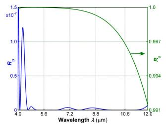
Fig. 6. (Color online) Reflectances  $R_p$  and  $R_s$  of ZnTe 1-D PCL of thickness  $d=10\,\mu\text{m},~f=0.604,$  embedded in ZnS cube, for incident p- and s-polarized light, plotted versus wavelength  $\lambda$ , for  $4\leq\lambda\leq12\,\mu\text{m}.~R_p$  exhibits interference oscillations, whereas  $R_s$  decreases monotonically as  $\lambda$  increases.
