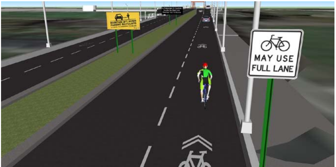
Better signage and more shared-lane striping
