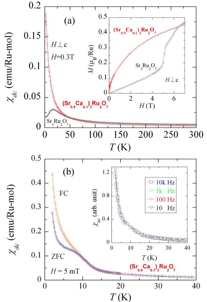
FIG. 2. (Color online) (a) dc magnetic susceptibility measured at 0.3 T for  $\text{Sr}_3\text{Ru}_2\text{O}_7$  and  $(\text{Sr}_{0.9}\text{Ca}_{0.1})_3\text{Ru}_2\text{O}_7$ . (Inset) The magnetization as a function of field at 2 K. (b) dc magnetic susceptibility measured at 5 mT for  $(\text{Sr}_{0.9}\text{Ca}_{0.1})_3\text{Ru}_2\text{O}_7$ . (Inset) The ac magnetic susceptibility measured at various frequencies for  $(\text{Sr}_{0.9}\text{Ca}_{0.1})_3\text{Ru}_2\text{O}_7$ .
