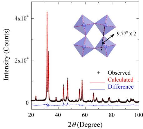
FIG. 1. (Color online) Observed (open circles), calculated (solid line), and different (bottom of the figure) intensities of powder diffraction pattern of the  $(\text{Sr}_{0.9}\text{Ca}_{0.1})_3\text{Ru}_2\text{O}_7$  sample at room temperature.  $R_{\text{wp}}=5.86\%$ ,  $R_p=4.33\%$ , and  $\chi^2=5.683$ . The inset shows the schematic of the octahedron rotation of  $\text{RuO}_6$ .
