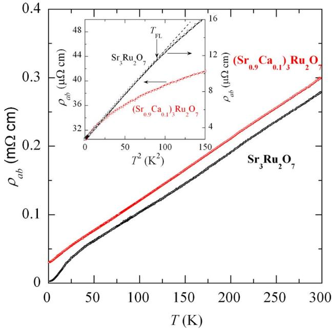
FIG. 3. (Color online) In-plane resistivity as a function of temperature for  $(\text{Sr}_{0.9}\text{Ca}_{0.1})_3\text{Ru}_2\text{O}_7$  and  $\text{Sr}_3\text{Ru}_2\text{O}_7$ . (Inset)  $\rho_{ab}$  vs  $T^2$  at low temperatures.
