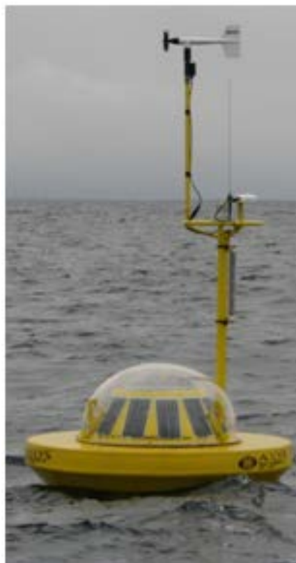
Figure 3. Close-up picture of a solar powered WatchMate™ Buoy.
