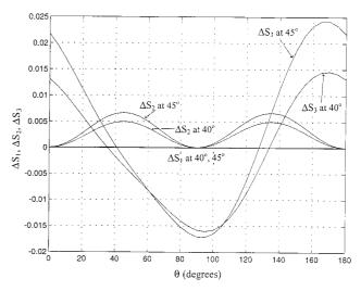
Fig. 16. Stokes parameters  $\Delta S_k$  (k=1,2,3) as functions of the longitude angle  $\theta$  obtained by use of a coated ZnS–SiO<sub>2</sub>–Ag parallel slab at  $\lambda=633$  nm and angles of incidence of  $\varphi_0=40^\circ,50^\circ$ . The thickness of the ZnS thin-film coating is 70 nm.
