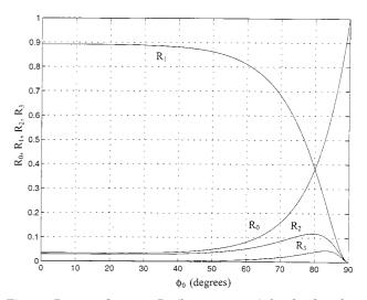
Fig. 4. Power reflectance  $R_k$  (k=0, 1, 2, 3) for the first four reflected orders as functions of the incidence angle  $\phi_0$  obtained by use of an uncoated SiO<sub>2</sub>–Ag parallel slab at  $\lambda=633$  nm.
