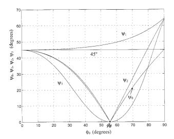
Fig. 2. Ellipsometric angle  $\psi_k$  (k=0,1,2,3) for the first four reflected orders as functions of the incidence angle  $\phi_0$  obtained by use of an uncoated SiO<sub>2</sub>–Ag parallel slab at  $\lambda=633$  nm.
