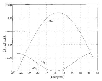
Fig. 13. Stokes parameters  $\Delta S_k$  (k=1,2,3) as functions of the latitude angle  $\epsilon$  obtained by use of a coated ZnS–SiO<sub>2</sub>–Ag parallel slab at  $\lambda=633$  nm, an angle of incidence of  $\phi_0=45^\circ$ , and a longitude angle of  $\theta=0$ . The thickness of the ZnS thin-film coating is 70 nm.
