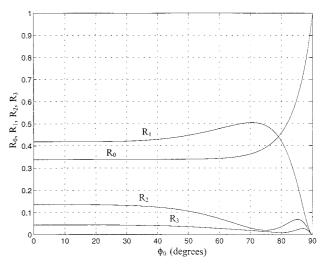
Fig. 6. Power reflectance  $R_k$  (k=0, 1, 2, 3) for the first four reflected orders as functions of the incidence angle  $\phi_0$  obtained by use of a coated ZnS–SiO<sub>2</sub>–Ag parallel slab at  $\lambda=633$  nm. The thickness d of the ZnS thin-film coating is 70 nm.
