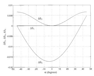
Fig. 15. Stokes parameters  $\Delta S_k$  (k=1,2,3) as functions of the latitude angle  $\epsilon$  obtained by use of a coated ZnS–SiO<sub>2</sub>–Ag parallel slab at  $\lambda=633$  nm, an angle of incidence of  $\phi_0=45^\circ$ , and a longitude angle of  $\theta=90^\circ$ . The thickness of the ZnS thin-film coating is 70 nm.
