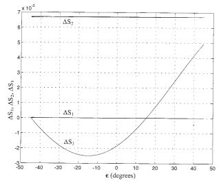
Fig. 14. Stokes parameters  $\Delta S_k$  (k=1,2,3) as functions of the latitude angle  $\epsilon$  obtained by use of a coated ZnS–SiO<sub>2</sub>–Ag parallel slab at  $\lambda=633$  nm, an angle of incidence of  $\phi_0=45^\circ$ , and a longitude angle of  $\theta=45^\circ$ . The thickness of the ZnS thin-film coating is 70 nm.
