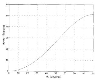
Fig. 3. Ellipsometric parameter  $\Delta_1-\Delta_3$  as a function of the angle of incidence  $\varphi_0$  obtained by use of an uncoated SiO\_2–Ag parallel slab at  $\lambda=633$  nm.
