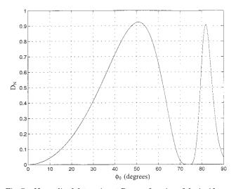
Fig. 7. Normalized determinant  $D_N$  as a function of the incidence angle  $\phi_0$  obtained by use of a coated ZnS–SiO<sub>2</sub>–Ag parallel slab at  $\lambda=633$  nm. The thickness d of the ZnS thin-film coating is 70 nm.
