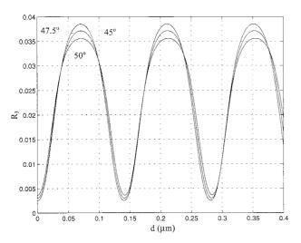
Fig. 9. Power reflectance  $R_k$  (k=0,1,2,3) for the first four reflected orders as functions of the coating thickness d obtained by use of a coated ZnS–SiO<sub>2</sub>–Ag parallel slab at  $\lambda=633$  nm. The angles of incidence are  $\phi_0=45^\circ,47.5^\circ,50^\circ.$
