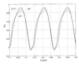
Fig. 10. Normalized determinant  $D_N$  as a function of the coating thickness d obtained by use of a coated ZnS–SiO<sub>2</sub>–Ag parallel slab at  $\lambda = 633$  nm. The angles of incidence are  $\phi_0 = 45^{\circ}$ ,  $47.5^{\circ}$ ,  $50^{\circ}$ .
