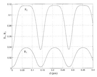
Fig. 8. Power reflectance  $R_k$  (k=2,3) for the second and the third reflected orders as functions of the coating thickness d obtained by use of a coated ZnS–SiO<sub>2</sub>–Ag parallel slab at  $\lambda=633$  nm and an angle of incidence of  $\phi_0=45^\circ$ .
