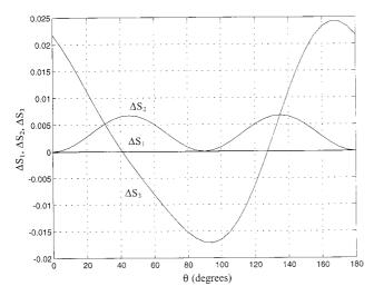
Fig. 11. Stokes parameters  $\Delta S_k$  (k=1,2,3) as functions of the longitude angle  $\theta$  obtained by used of a coated ZnS–SiO<sub>2</sub>–Ag parallel slab at  $\lambda=633$  nm and an angle of incidence of  $\varphi_0=45^\circ$ . The thickness of the ZnS thin-film coating is 70 nm.
