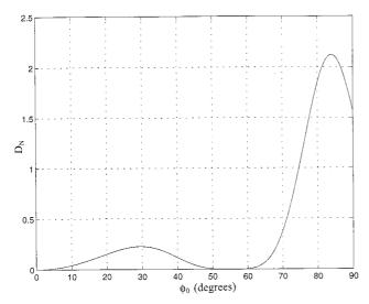
Fig. 5. Normalized determinant  $D_N$  as a function of the incidence angle  $\phi_0$  obtained by use of an uncoated SiO<sub>2</sub>–Ag parallel slab at  $\lambda$  = 633 nm.
