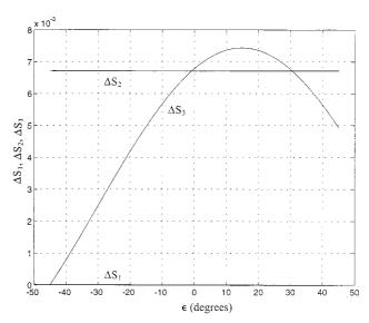
Fig. 12. Stokes parameters  $\Delta S_k$  (k=1,2,3) as functions of the latitude angle  $\epsilon$  obtained by used of a coated ZnS–SiO<sub>2</sub>–Ag parallel slab at  $\lambda=633$  nm, an angle of incidence of  $\phi_0=45^\circ$ , and a longitude angle of  $\theta=-45^\circ$ . The thickness of the ZnS thin-film coating is 70 nm.
