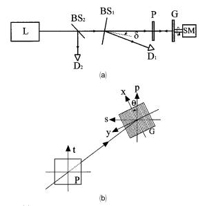
Fig. 1. (a) Experimental setup of the NIRSE: L, light source; BS<sub>1</sub>, BS<sub>2</sub>, beam splitters; D<sub>1</sub>, D<sub>2</sub>, silicon photodetectors; P, Glan—Thompson polarizer; G, grating sample; SM, stepping motor. (b) Relative position of the rotating x-y and space-fixed p-s Cartesian coordinate systems. P and G are the same as in (a).
