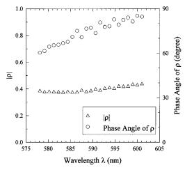
Fig. 4. Absolute value and phase angle of  $\rho$  as a function of wavelength  $\lambda$  for a 600-grooves/mm aluminum-coated grating.<sup>11</sup>
