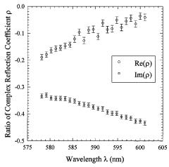
Fig. 3.  $Re(\rho)$  and  $Im(\rho)$  as functions of wavelength  $\lambda$  for a 600-grooves/mm aluminum-coated grating. <sup>11</sup> The standard deviation of the measurement varies from 0.015 to 0.025 when a dye laser is used as the light source.
