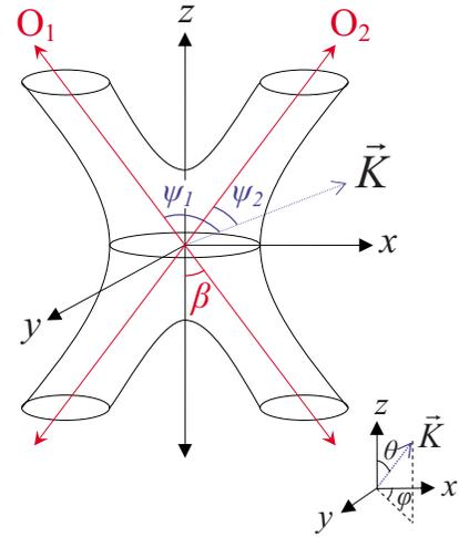
FIG. 1. (Color online) Bertin surfaces of constant phase difference between ordinary and extraordinary rays for an optically biaxial crystal.
