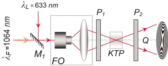
FIG. 2. (Color online) Optical setup for conoscopic interferometry and SHG generation. M1, P1, P2, and FO are, respectively, a mirror, polarizer, analyzer, and the focusing-optics. Orientation of P2 is orthogonal to P1. Q is the axis of the conoscopic-interferometer.  $\lambda_L$  and  $\lambda_F$  are the conoscopic-illumination-wavelength and the fundamental-pump-wavelength, respectively. The two laser-beams should be collinear. M1, P1, P2, and FO should be mounted on a foldable-mirror mount.
