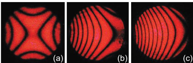
FIG. 3. (Color) Observed conoscopic interferograms for  $x$ -cut KTP at goniometer-rotation-angles of (a)  $0^\circ$ , (b)  $5^\circ$ , and (c)  $10^\circ$ .
