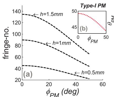
FIG. 7. (Color online) Calculated fringe-numbers showing the intersection of dark-fringes on the conoscopic interferogram to Type-I PM directions for an  $z$ -cut KTP. The interferogram is calculated for an illuminating wavelength of 633 nm and the PM directions correspond to a fundamental-wavelength of 1064 nm. (a) Fringe-number corresponding to type-I PM directions, for various crystal thicknesses. (b) Type-I PM.
