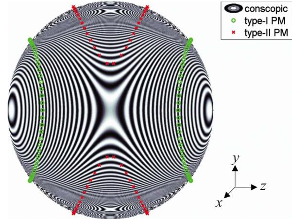
FIG. 4. (Color online) Calculated conoscopic interferogram for a  $x$ -cut KTP, for a illumination wavelength,  $\lambda=633$  nm. Corresponding projections for type-I and type-II PM on the  $z$ - $y$  plane, are shown. PM directions are calculated for a fundamental wavelength of 1064 nm. A thickness,  $h=0.5$  mm was chosen for the purpose of illustration.
