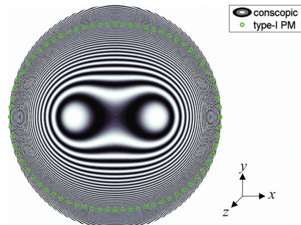
FIG. 5. (Color online) Calculated conoscopic-interferogram for a  $z$ -cut KTP, for a illumination wavelength,  $\lambda=633$  nm. Corresponding projections for type-I PM on the  $x$ - $y$  plane, are shown. PM directions are calculated for a fundamental wavelength of 1064 nm. A thickness,  $h=0.5$  mm was chosen for the purpose of illustration.
