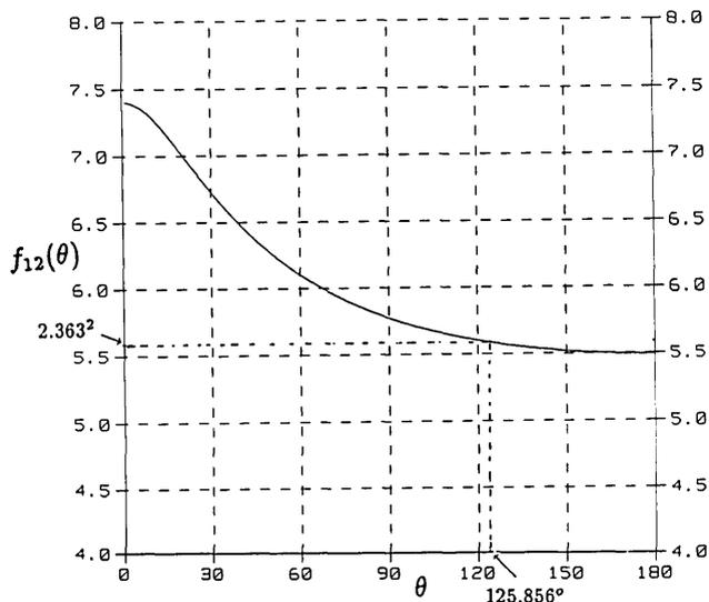
Fig. 9. Function  $f_{12}(\theta)$  of Eq. (51) plotted vs  $\theta$  for the pseudo-Brewster angles of external and internal reflection,  $\phi_{pB1} = 66.4323^\circ$  and  $\phi_{pB2} = 40.1148^\circ$ , of a TiN film on a ZnS substrate. The point of intersection of the curve with a horizontal line drawn at an ordinate =  $2.363^2$  gives the argument  $\theta (= 125.856^\circ)$  of complex  $\epsilon$  of the TiN film.
