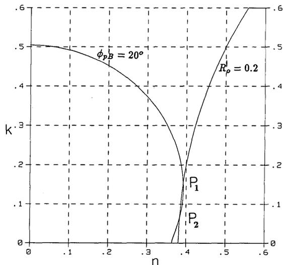
Fig. 7. In the domain of fractional optical constants, an iso- $R_o$  contour ( $R_o = 0.20$ ) may intersect an iso- $\phi_{pB}$  contour ( $\phi_{pB} = 20^\circ$ ) at two points  $P_1$  and  $P_2$  that specify two valid solution pairs  $(n, k)$  at  $P_1$  and  $P_2$ .
