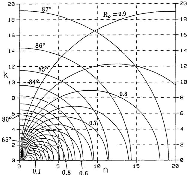
Fig. 5. Similar to Fig. 4 except that the constant values of  $\phi_{pB}$  are  $65^\circ, 70^\circ, 73^\circ, 75^\circ, 77^\circ, 79^\circ,$  and  $80^\circ\text{--}87^\circ$  in steps of  $1^\circ$ . ( $R_o$  is in the range from 0.05 to 0.90 in steps of 0.05, as in Fig. 4). Again this nomogram serves as an aid in solving the  $(R_o, \phi_{pB}) \rightarrow (n, k)$  inversion problem.
