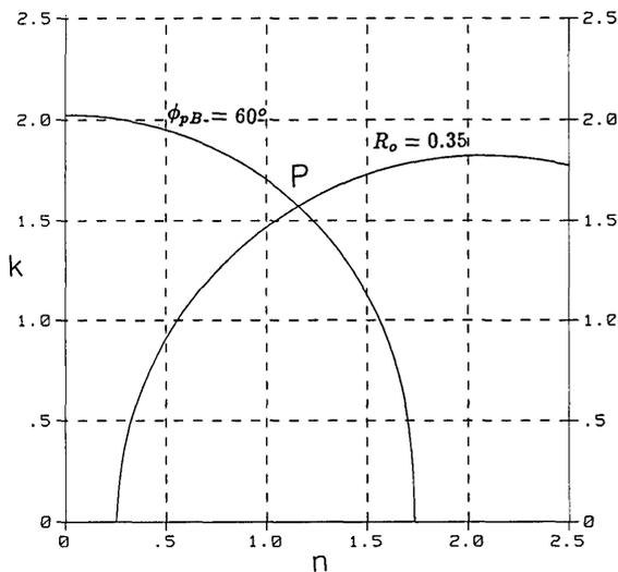
Fig. 6. An iso- $R_o$  contour ( $R_o = 0.35$ ) generally intersects an iso- $\phi_{pB}$  contour ( $\phi_{pB} = 60^\circ$ ) at one point  $P$  that specifies a unique solution pair  $(n, k)$  at  $P$ .
