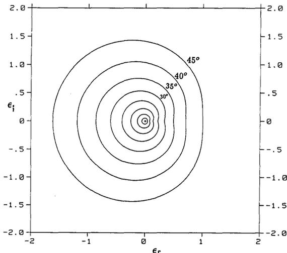
Fig. 1. Contours of constant pseudo-Brewster angle  $\phi_{PB}$  in the complex  $\epsilon$  plane for angles  $\phi_{PB}$  from 5° to 45° in 5° steps. Each contour is symmetrical with respect to the real axis.
