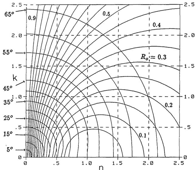
Fig. 4. Families of iso- $R_o$  and iso- $\phi_{pB}$  contours in the  $nk$  plane.  $R_o$  is the normal incidence reflectance and assumes values from 0.05 to 0.90 in steps of 0.05.  $\phi_{pB}$  is the pseudo-Brewster angle and takes values from  $5^\circ$  to  $65^\circ$  in steps of  $5^\circ$ . This nomogram can be used to find an approximate solution for the optical constants  $(n,k)$  given a measured set  $(R_o, \phi_{pB})$ .
