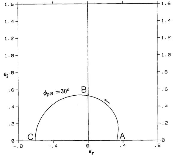
Fig. 3. An iso- $\phi_{pB}$  contour in the upper half of the complex  $\epsilon$  plane.  $A$ ,  $B$ , and  $C$  are the points of intersection of the contour with the positive real axis, imaginary axis, and negative real axis, respectively. The arrow indicates the direction in which the minimum reflectance (at  $\phi_{pB}$ ) increases monotonically from 0 at  $A$  to 1 at  $C$ .
