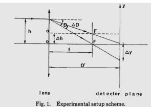
using a Schottky-barrier surface position-sensitive detector
