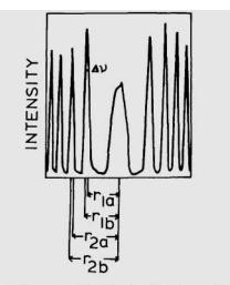
Fig. 4. Single-pulse spectral distribution of the laser output obtained as a microdensitometer trace of a photoplate.
