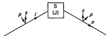
FIG. 1. A beam of polarized light interacts with a linear nondepolarizing optical sample  $S$  with Jones matrix  $J$ .  $ps$  is a reference Cartesian coordinate system defined in the same manner for both the input ( $i$ ) and output ( $o$ ) beams.
