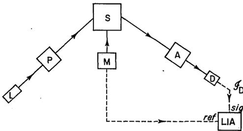
FIG. 2. A general ellipsometer arrangement with arbitrary polarizing ( $P$ ) and analyzing ( $A$ ) optics.  $S$  is the sample under measurement by MGE, and  $M$  is the source of modulation applied to  $S$ . The signal output  $s_D$  of the photodetector  $D$  can be measured by a lock-in amplifier LIA, which receives its reference signal from  $M$ .  $L$  represents the light source.
