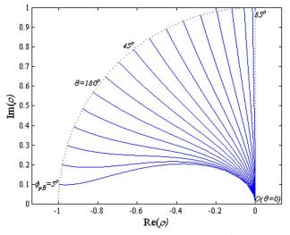
Fig. 8. Complex-plane trajectories of the ratio  $\rho = r_p/r_s$  at discrete values of the PBA  $\phi_{pB}$  from 5° to 85° in equal steps of 5° as  $\theta = -\arg(\varepsilon)$  covers the full range  $0^\circ \le \theta \le 180^\circ$ .
