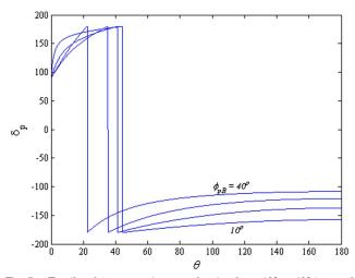
Fig. 5. Family of  $\delta_p$  versus  $\theta$  curves for  $\phi_{pB}$  from 10° to 40° in equal steps of 10°. Both  $\theta$  and  $\delta_p$  are in degrees.
