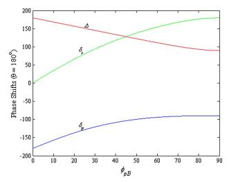
Fig. 4. Total reflection phase shifts  $\delta_p$ ,  $\delta_s$ , and  $\Delta = \delta_p - \delta_s + 360^\circ$  at the interface between a dielectric and plasmonic medium in the limit as  $\theta \to 180^\circ$  ( $\varepsilon_i = 0$ ,  $\varepsilon_r < 0$ ) are plotted as a functions of  $\phi_{pB}$ . All angles are in degrees.
