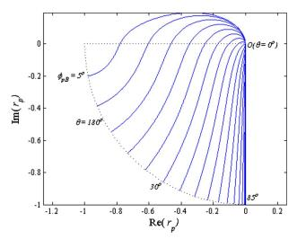
Fig. 1. Complex-plane trajectories of  $r_p$  at discrete values of the PBA  $\phi_{pB}$  from 5° to 85° in equal steps of 5° as  $\theta = -\arg(\varepsilon)$  covers the full range  $0^{\circ} \le \theta \le 180^{\circ}$ .
