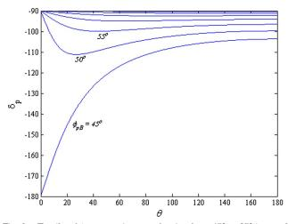
Fig. 6. Family of  $\delta_p$  versus  $\theta$  curves for  $\phi_{pB}$  from 45° to 85° in equal steps of 5°. Both  $\theta$  and  $\delta_p$  are in degrees.
