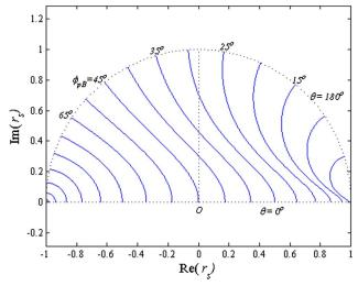
Fig. 7. Complex-plane contours of  $r_s$  at discrete values of the PBA  $\phi_{pB}$  from 5° to 85° in equal steps of 5° as  $\theta = -\arg(\varepsilon)$  covers the full range from 0° to 180°.
