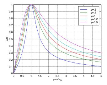
**FIGURE 2.** Relationship between the normalized impedance magnitude Z/R and the normalized frequency  $\gamma = \omega/\omega_o$  for the circuit of Fig. 1.
