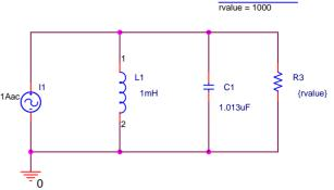
**FIGURE 3.** PSpice schematic diagram of the parallel *RLC* circuit used in the simulations.
