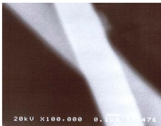
**Figure 2.7(b)** SEM image of higher magnification of gold nanowires
