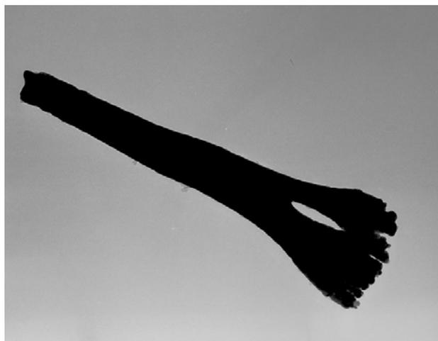
**Figure 2.11** TEM image of the gold nanowire fabricated by pulsed electrochemical method
