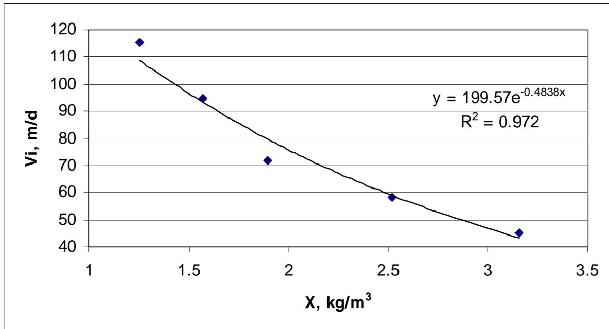
**Figure E-12 Field Data and Fitted Exponential Equation for Zone Settling**
