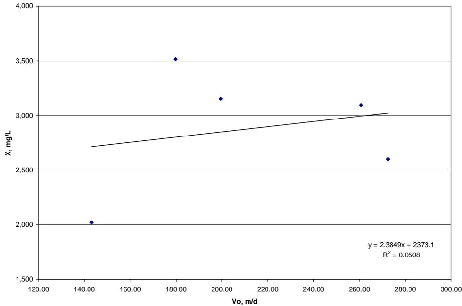
Figure 4.10 Relationship between the MLSS concentrations and the empirical parameter  $V_0$  during a HRT of 30 min
