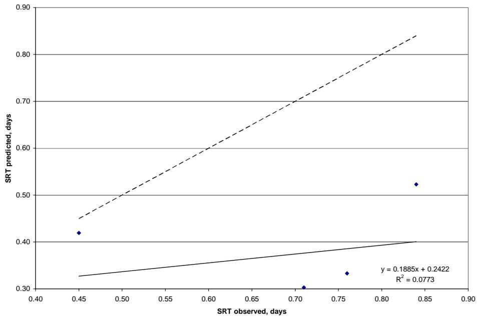
Figure 4.6 Relationship between the SRT Observed in the Field and the SRT Predicted during a HRT of 30 min
