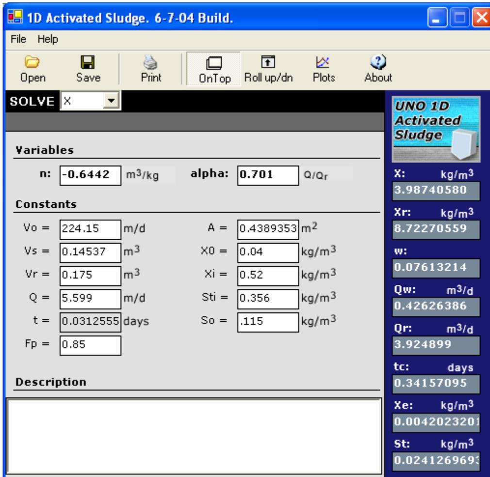
Figure D-6 Data predicted by the UNO 1D Activated Sludge Model, HRT 45 min (Day 6)
