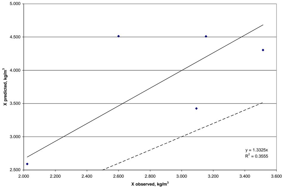
Figure 4.2 Relationship between the MLSS Concentration Observed in the Field and the MLSS Concentration Predicted during a HRT of 30 min
