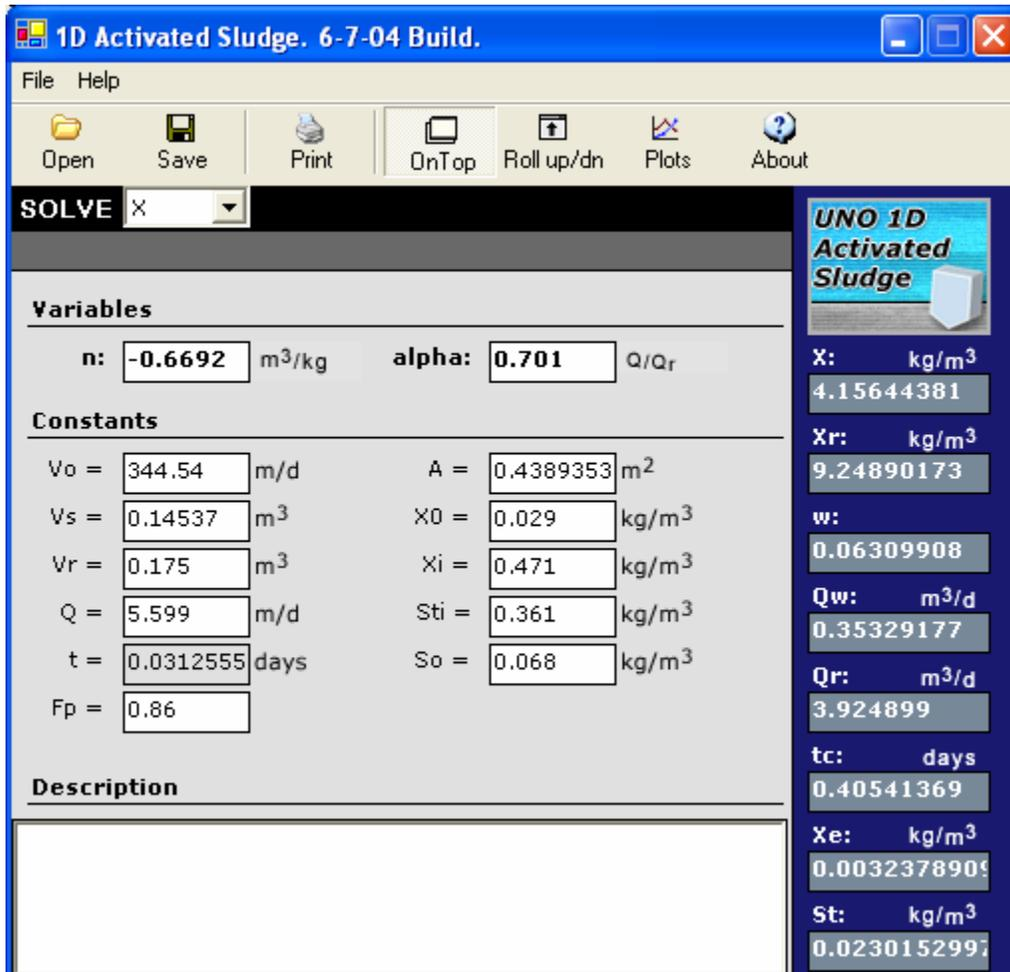
Figure D-5 Data predicted by the UNO 1D Activated Sludge Model, HRT 45 min (Day 5)
