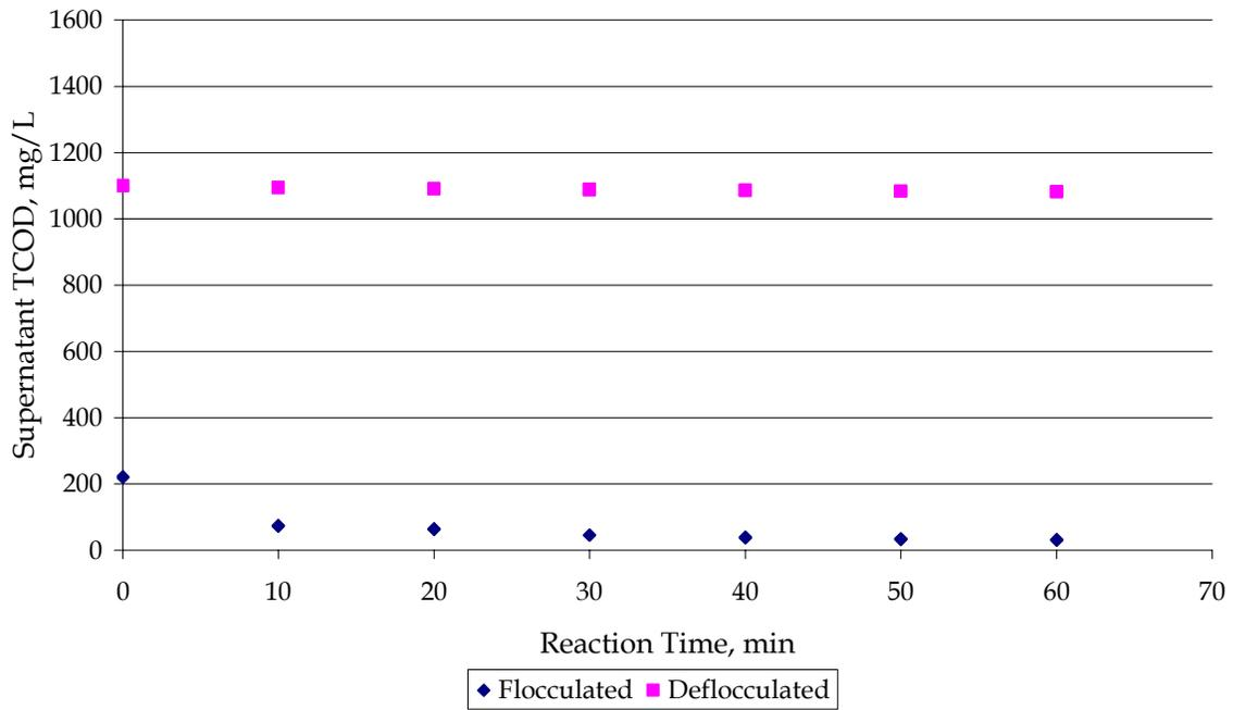
Figure 2.3 Effect of Bioflocculation on TCOD Removal. (La Motta et al., 2004)
