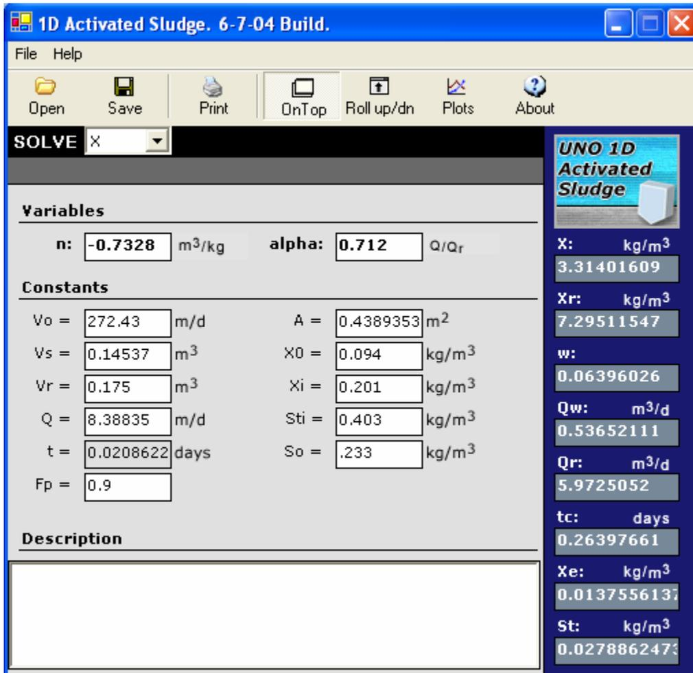
Figure D-10 Data predicted by the UNO 1D Activated Sludge Model, HRT 30 min (Day 2)
