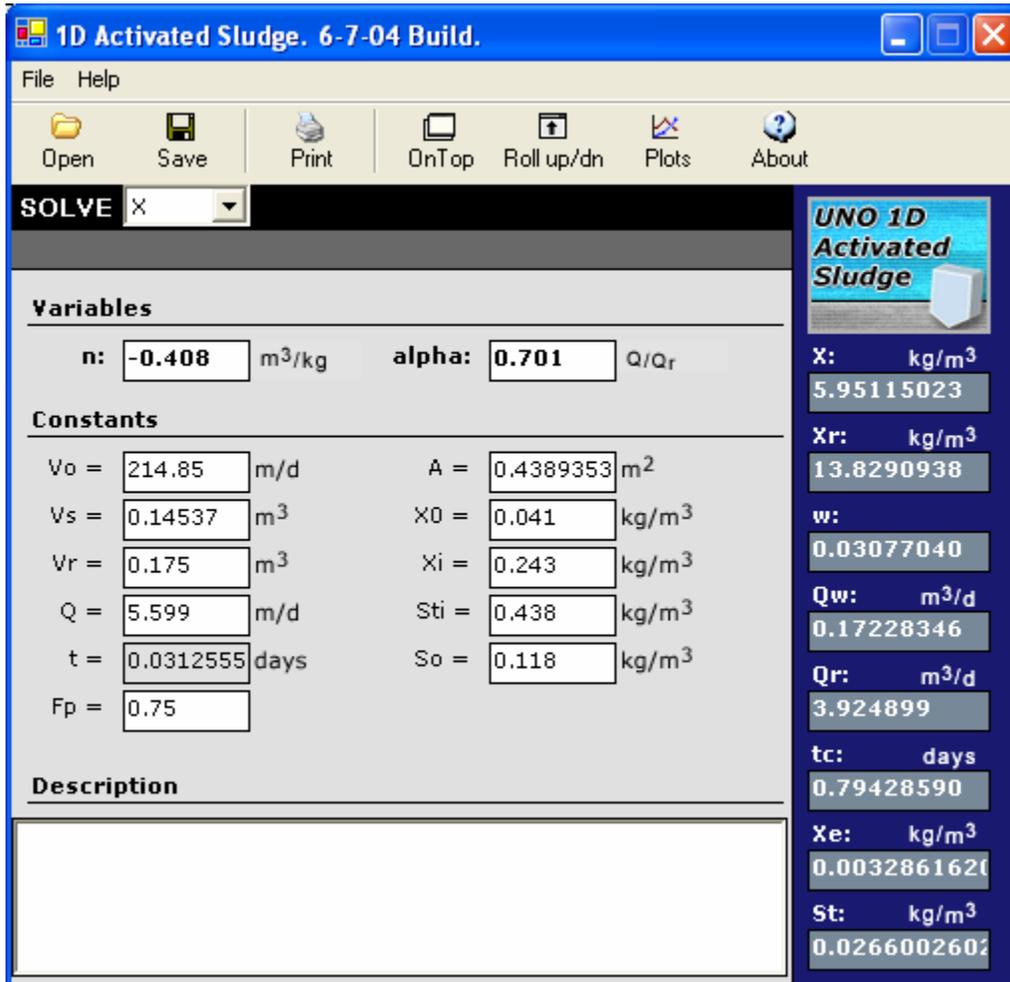
Figure D-8 Data predicted by the UNO 1D Activated Sludge Model, HRT 45 min (Day 8)
