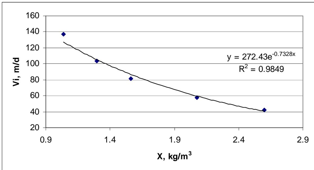
**Figure E-10 Field Data and Fitted Exponential Equation for Zone Settling**
