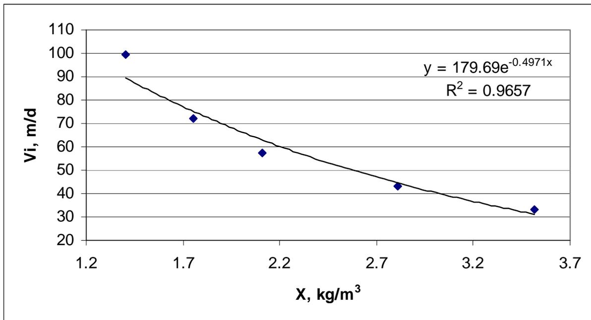
**Figure E-13 Field Data and Fitted Exponential Equation for Zone Settling**
