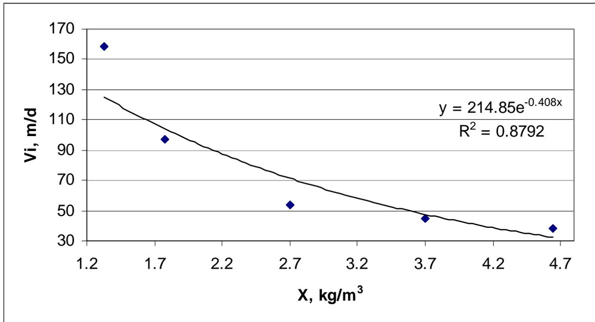
**Figure E-8 Field Data and Fitted Exponential Equation for Zone Settling**
