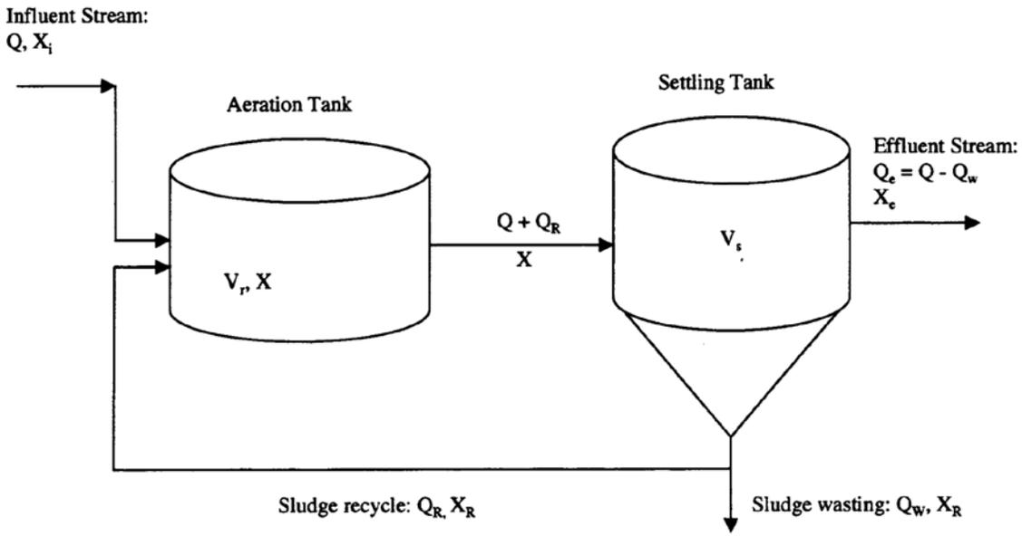
Figure 2.6 Complete-Mix Aerator Tank with Sludge Recycle. (La Motta, 2004)
