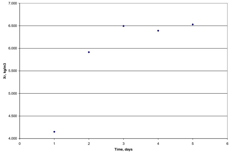
Figure 4.14 Recycled Sludge Concentration vs. Time during HRT of 30 min
