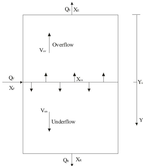
Figure 2.1 Flow Scheme of the one-dimensional continuous-flow settling tank approach. (Ekama et al., 1997)
