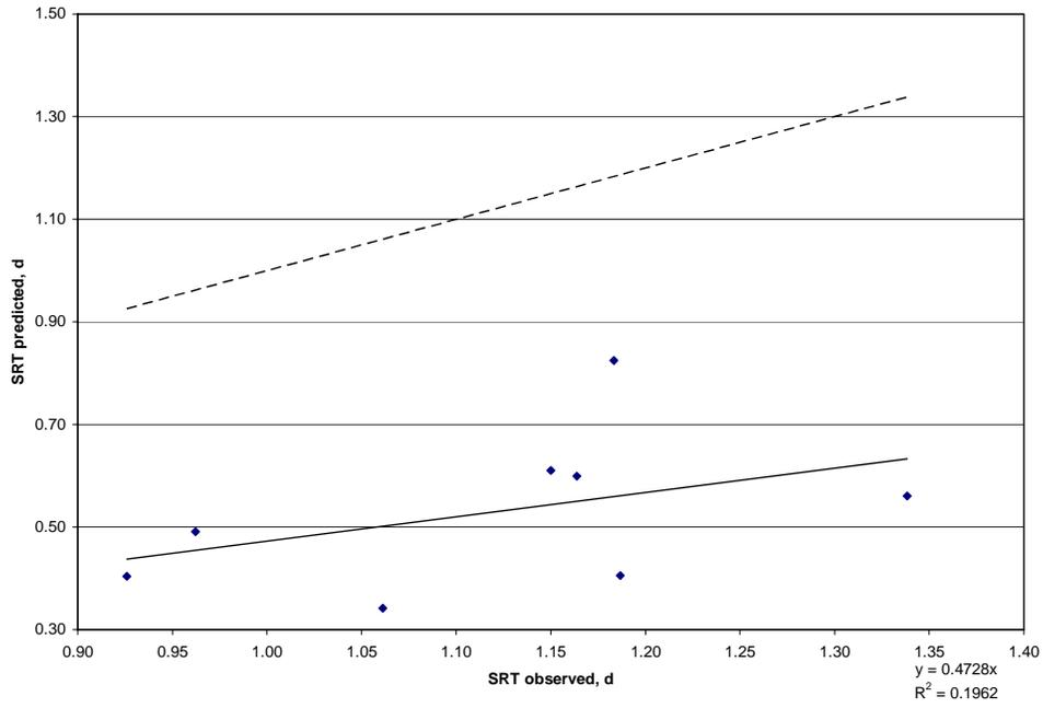
Figure 4.5 Relationship between the SRT Observed in the Field and the SRT predicted during a HRT of 45 min
