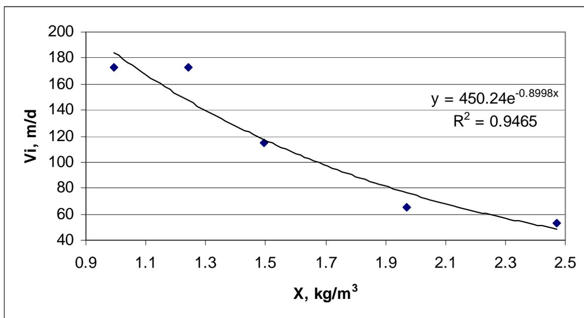
**Figure E-3 Field Data and Fitted Exponential Equation for Zone Settling**
