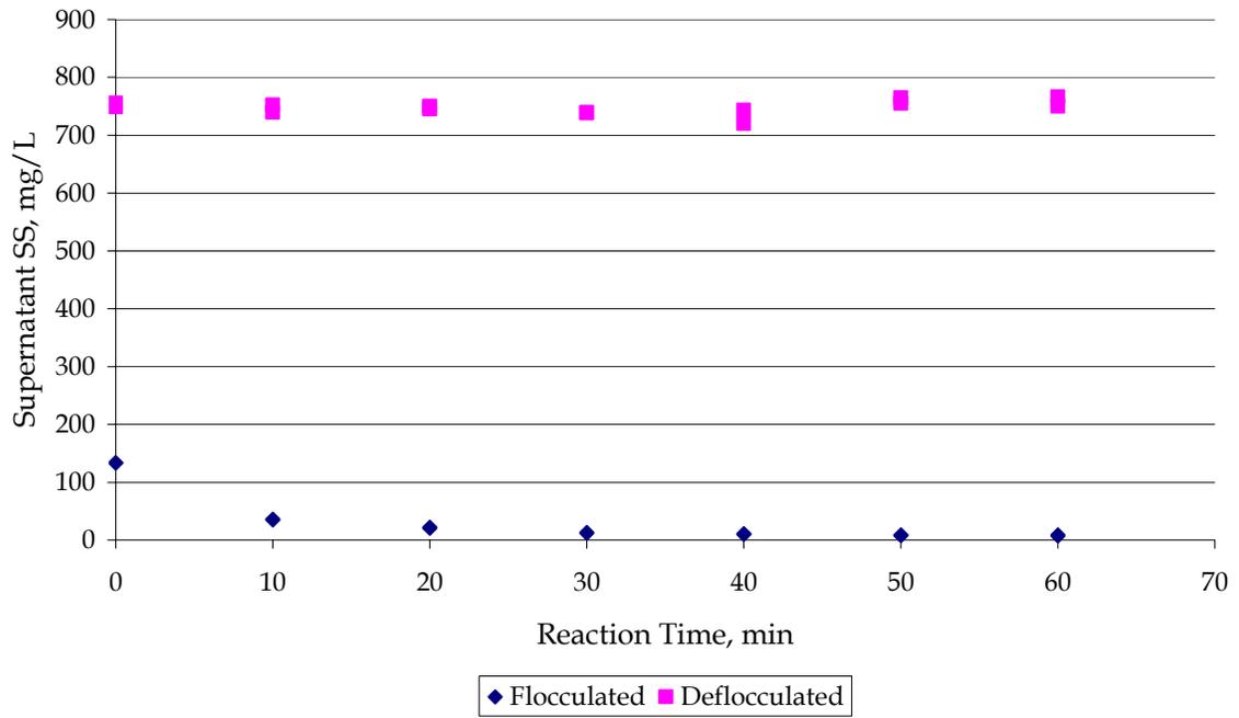
Figure 2.2 Effect of Bioflocculation on Supernatant SS Removal. (La Motta et al., 2004)
