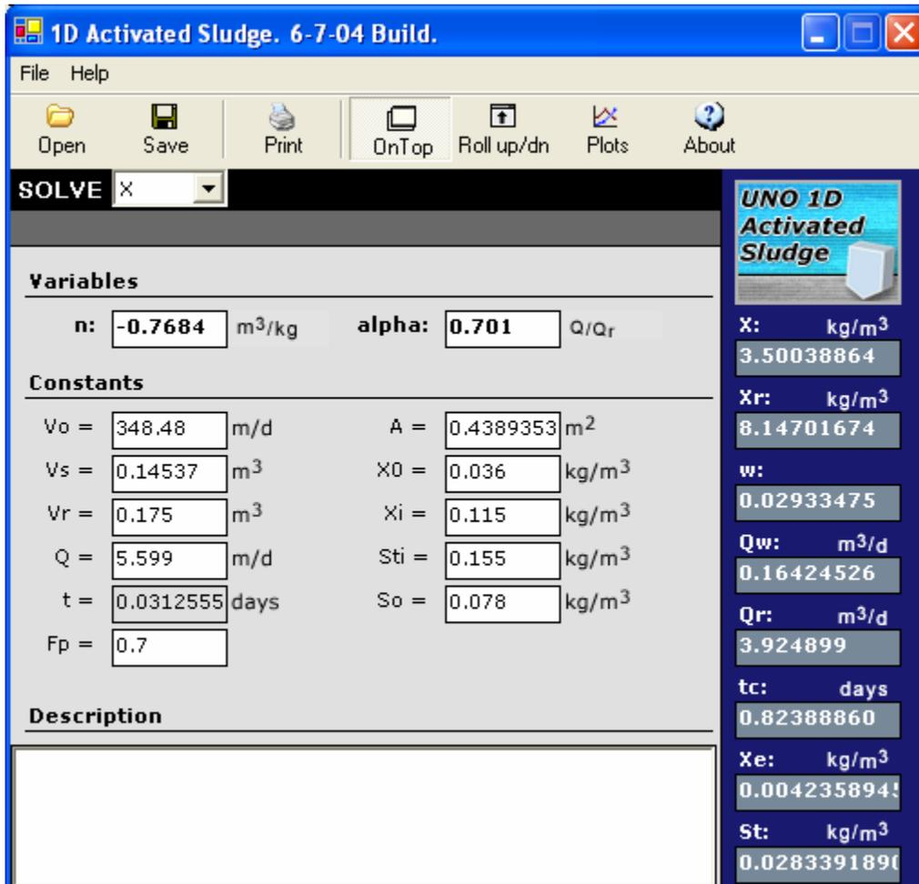
Figure D-4 Data predicted by the UNO 1D Activated Sludge Model, HRT 45 min (Day 4)
