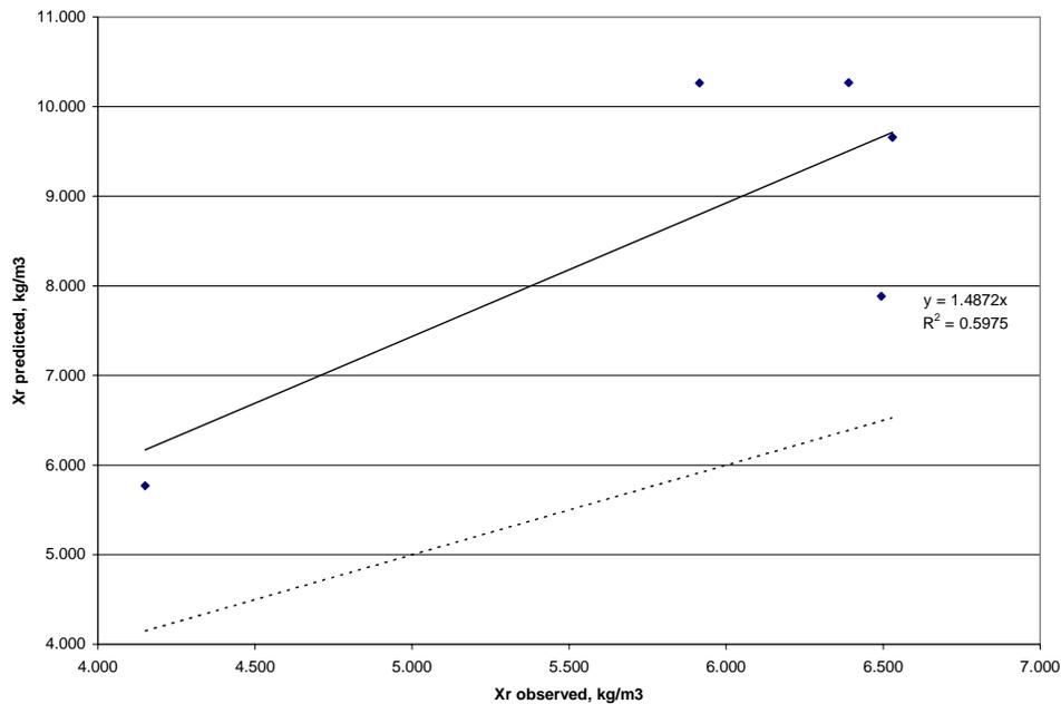
Figure 4.4 Relationship between the  $X_R$  Concentration Observed in the Field and the  $X_R$  Concentration Predicted during a HRT of 30 min
