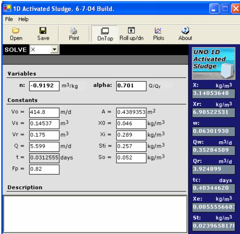
Figure D-1 Data predicted by the UNO 1D Activated Sludge Model, HRT 45 min (Day 1)
