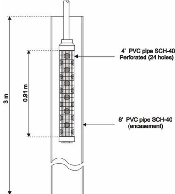
Figure 3.2 Straining Device (Padron 2004)
