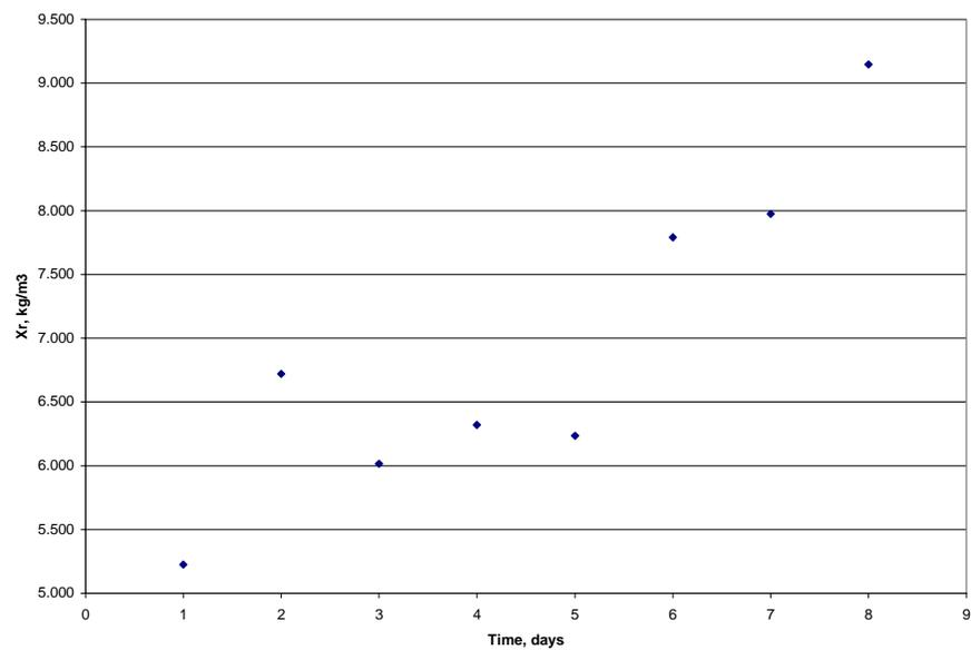
Figure 4.13 Recycled Sludge concentration vs. Time during HRT of 45 min
