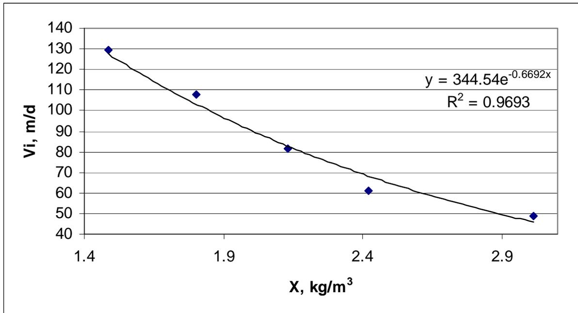
**Figure E-5 Field Data and Fitted Exponential Equation for Zone Settling**
