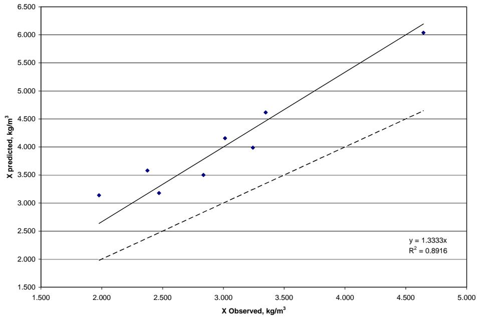
Figure 4.1 Relationship between the MLSS Concentration Observed in the Field and the MLSS Concentration Predicted during a HRT of 45 min
