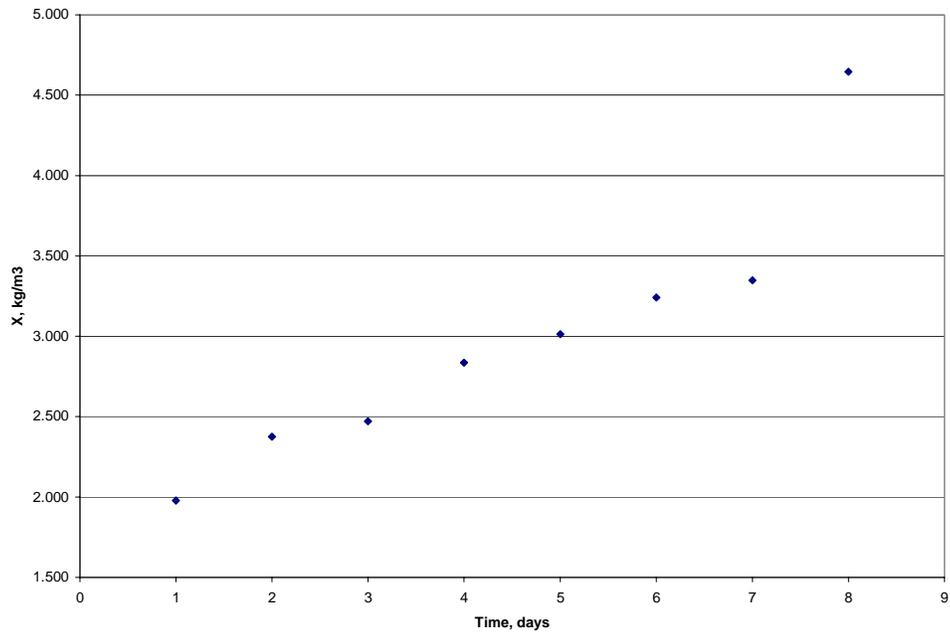
Figure 4.11 MLSS concentration vs. time during HRT of 45 min
