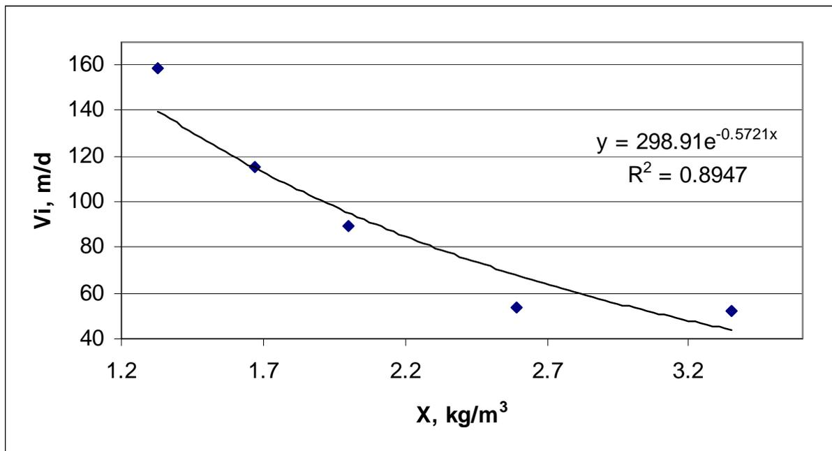
**Figure E-7 Field Data and Fitted Exponential Equation for Zone Settling**
