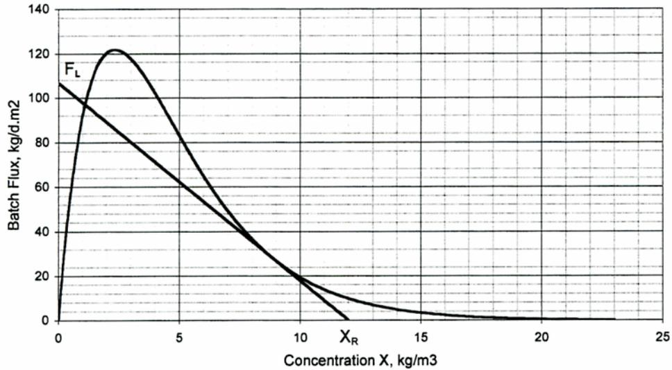
Figure 2.7 Graphical representation of the Limiting flux for settling tank design. (La Motta, 2004)
