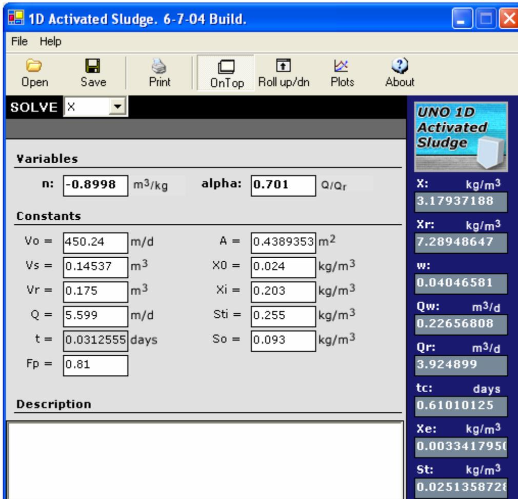
Figure D-3 Data predicted by the UNO 1D Activated Sludge Model, HRT 45 min (Day 3)
