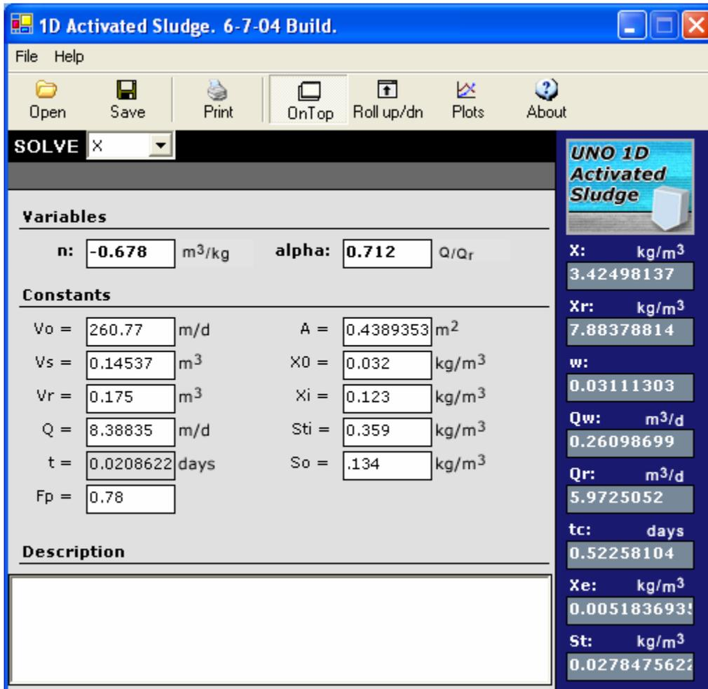
Figure D-11 Data predicted by the UNO 1D Activated Sludge Model, HRT 30 min (Day 3)
