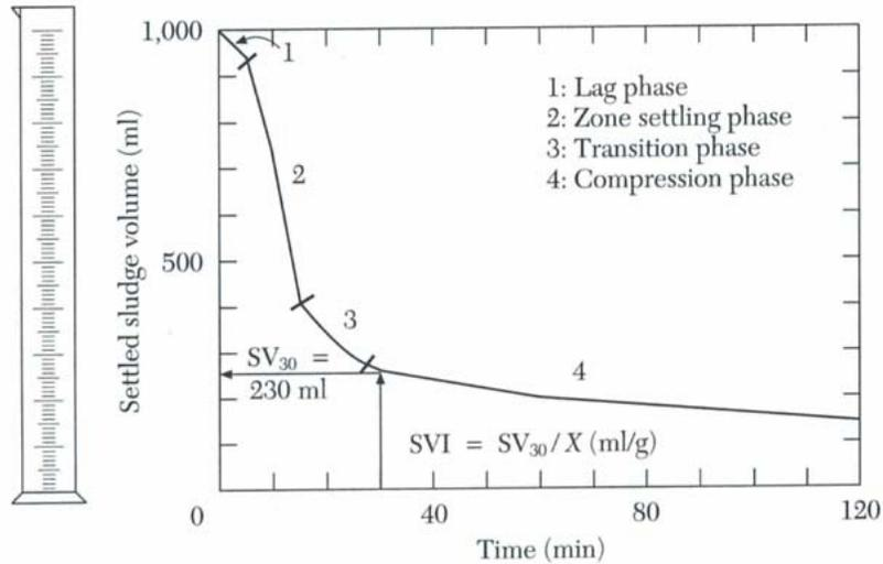
Figure 2.5 Plot of solid/liquid interface depth against the time in an unstirred measuring cylinder showing the appearance of the different stages of settlement at the solid/liquid interface (Ekama et al., 1997).
