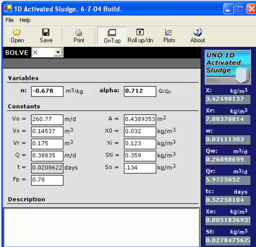
Figure D-12 Data predicted by the UNO 1D Activated Sludge Model, HRT 30 min (Day 4)
