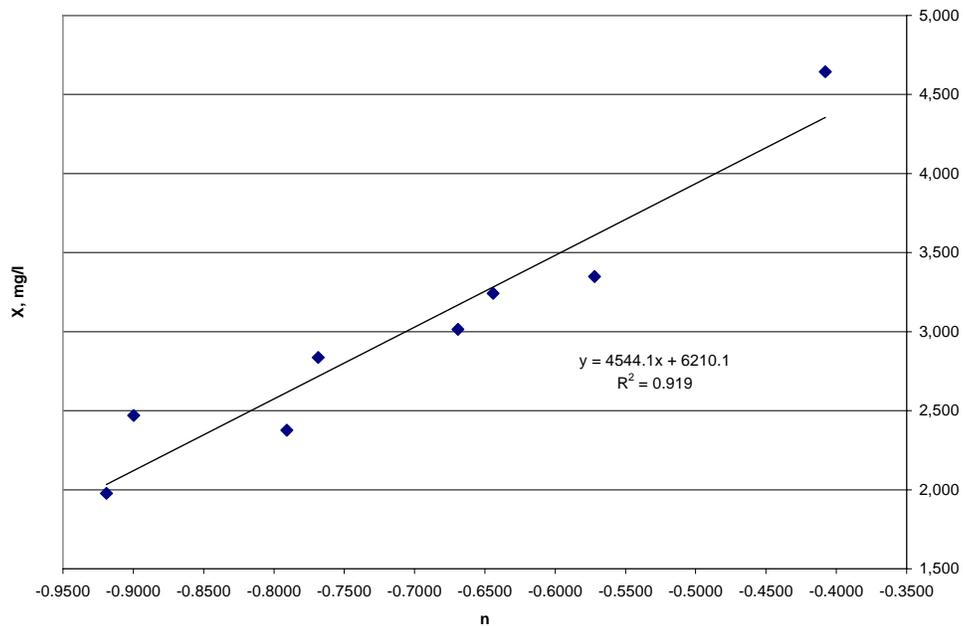
Figure 4.7 Relationship between the MLSS concentrations and the empirical parameter  $n$  during a HRT of 45 min
