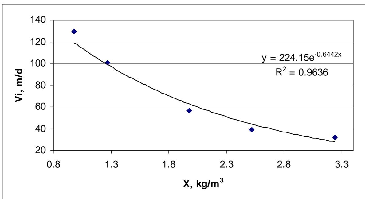
**Figure E-6 Field Data and Fitted Exponential Equation for Zone Settling**
