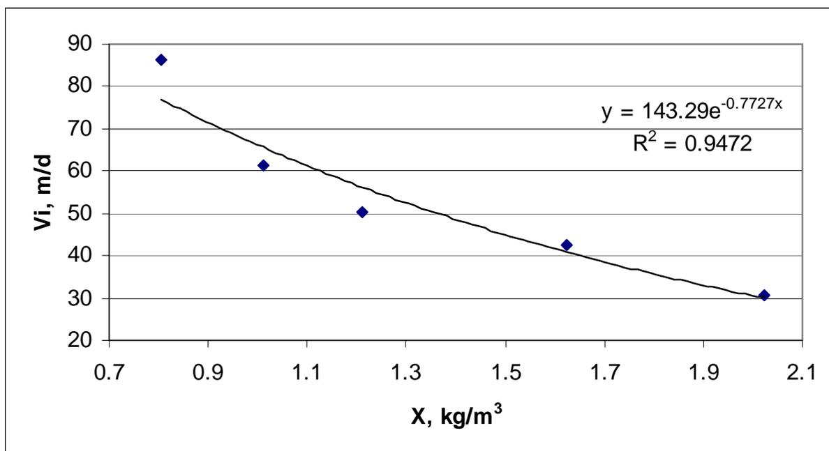
**Figure E-9 Field Data and Fitted Exponential Equation for Zone Settling**
