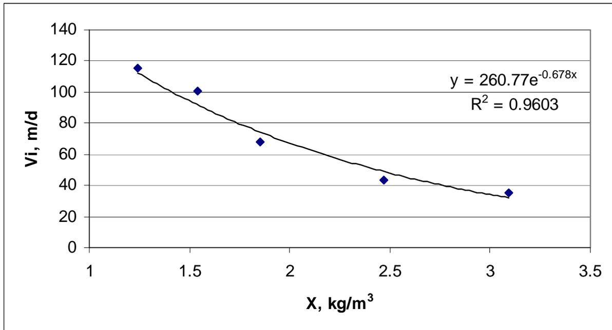
**Figure E-11 Field Data and Fitted Exponential Equation for Zone Settling**
