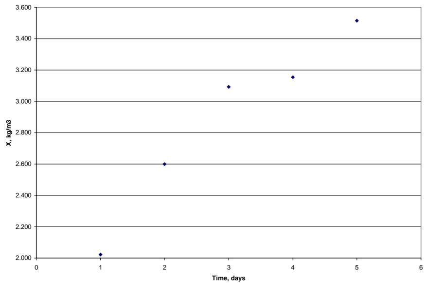
Figure 4.12 MLSS concentration vs. time during HRT of 30 min
