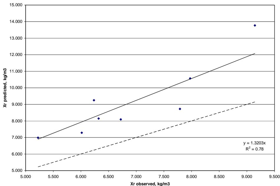
Figure 4.3 Relationship between the  $X_R$  Concentration Observed in the Field and the  $X_R$  Concentration Predicted during a HRT of 45 min
