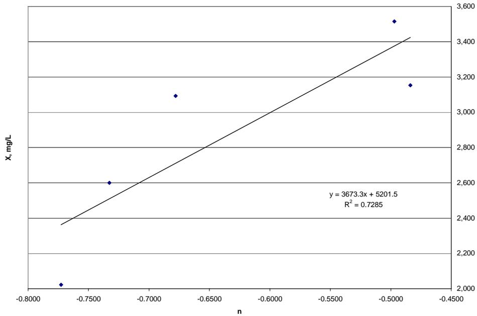
Figure 4.8 Relationship between the MLSS concentrations and the empirical parameter  $n$  during a HRT of 30 min
