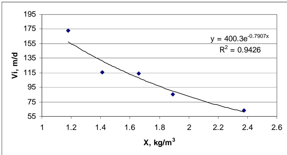
**Figure E-2 Field Data and Fitted Exponential Equation for Zone Settling**
