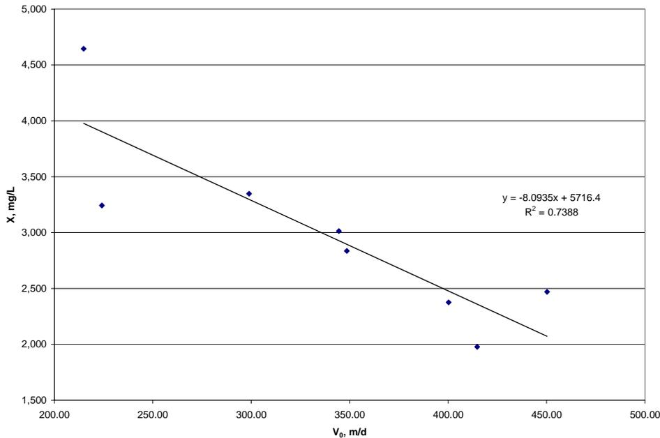
Figure 4.9 Relationship between the MLSS concentrations and the empirical parameter  $V_0$  during a HRT of 45 min
