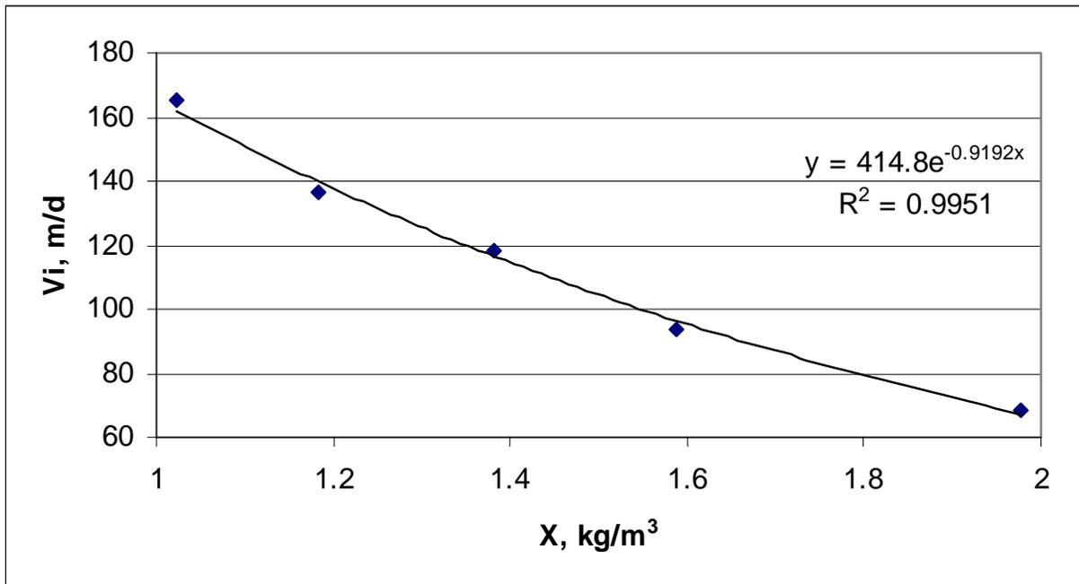
**Figure E-1 Field Data and Fitted Exponential Equation for Zone Settling**
