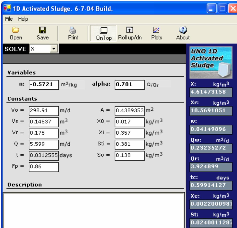
Figure D-7 Data predicted by the UNO 1D Activated Sludge Model, HRT 45 min (Day 7)
