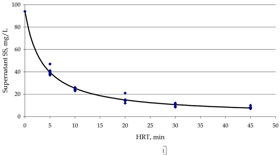
Figure 2.4 Effect of HRT on the Supernatant SS Removal. (La Motta et al., 2004)
