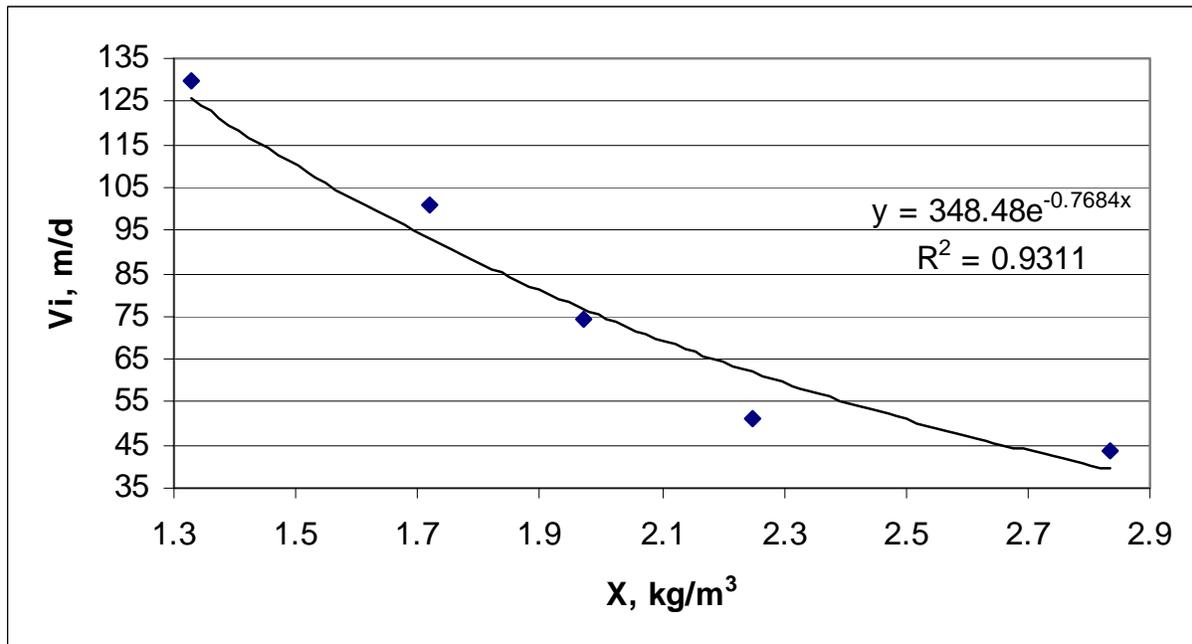
**Figure E-4 Field Data and Fitted Exponential Equation for Zone Settling**
