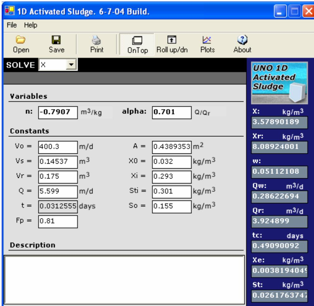
Figure D-2 Data predicted by the UNO 1D Activated Sludge Model, HRT 45 min (Day 2)
