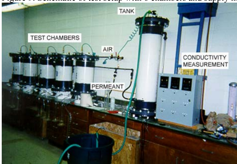
Figure 9. Schematic of test setup with 6 chambers and supply manifold
