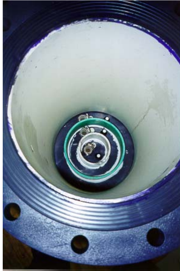
Figure 6. Photograph showing the center, middle and outer rings to separate the flow.
