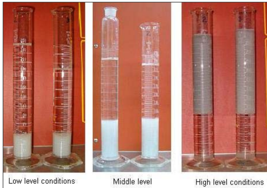
Figure 16. Treated water at three different current conditions after sedimentation /flotation.
