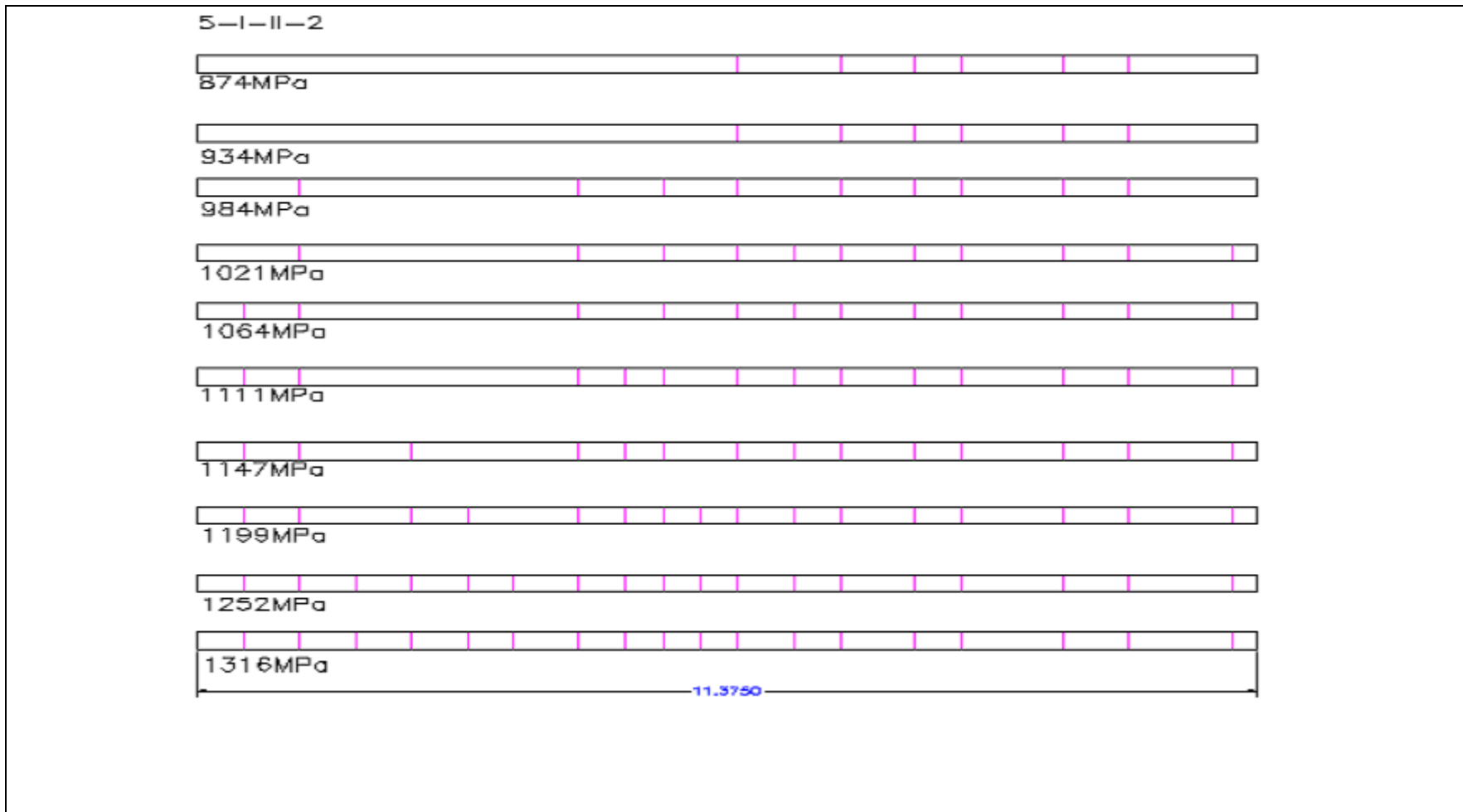
Figure 4.8 Schematics of Crack Propagation in Specimen 5-I-II-2.
