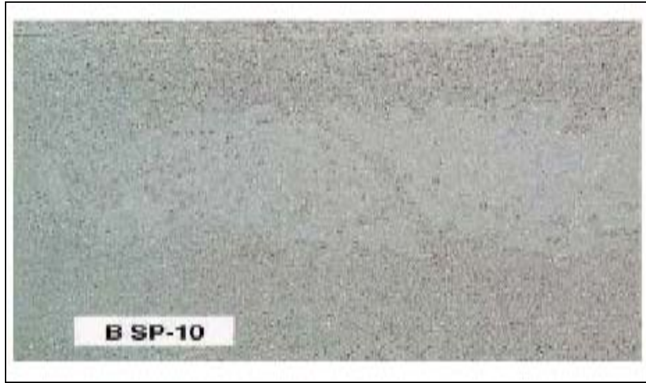
Figure 4 SSPC – SP10 Surface Finish, Source: The Society for Protective Coatings
