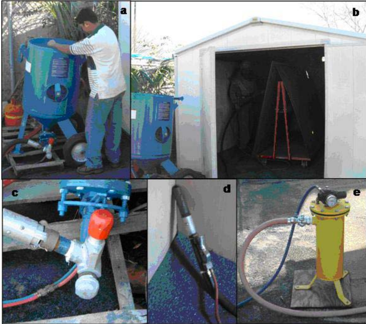
Figure 9 Blasting Equipment (a) Blast pot, (b) Blast chamber and test plates mounted on mobile cart, (c) Schmidt valve, (d) Bazooka #6 nozzle, (e) Secondary air supply filter
