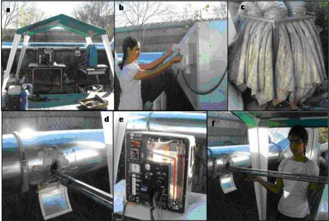
Figure 11 TPM Sampling Equipment (a) Stack sampling enclosure, (b) variable speed fan to vent particulate emissions, (c) particulate collection system, (d) stack and sampling port, (e) Stack sampling kit, (f) sampling in progress
