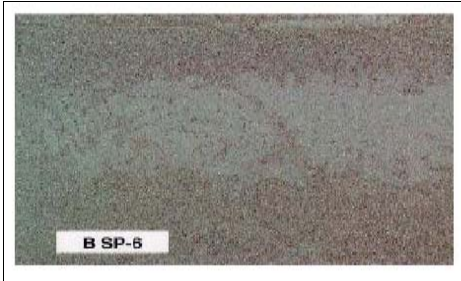
Figure 3 SSPC – SP6 Surface Finish, Source: The Society for Protective Coatings
