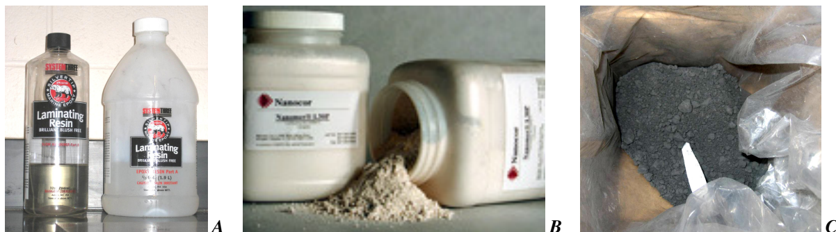
Figure 3.1: (A) epoxy part B and part A, (B) nanoclays 1 , (C) carbon nanofibers
