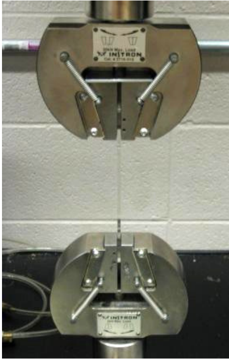
Figure 3.12: clamps with dog-bone specimen for tensile tests
