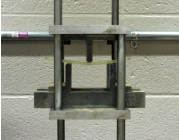
Figure 3.13: three point bending fixture with specimen for flexural tests
