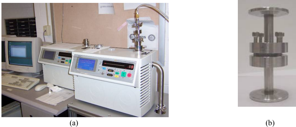
Figure 3.7 (a) Permeability set up (b) fixture with sample sandwiched between o-rings
