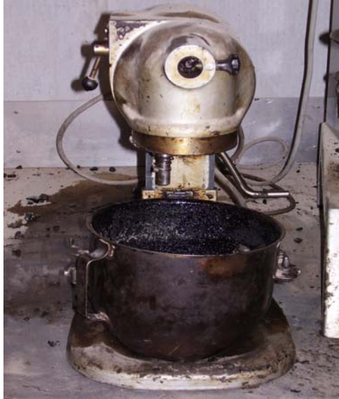
Fig 3.19: Mechanical Mixer and Mixing Bucket
