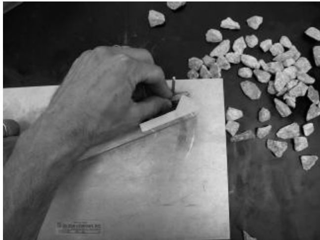
Figure 3.16: Testing Caliper Measuring the Flat Dimension
