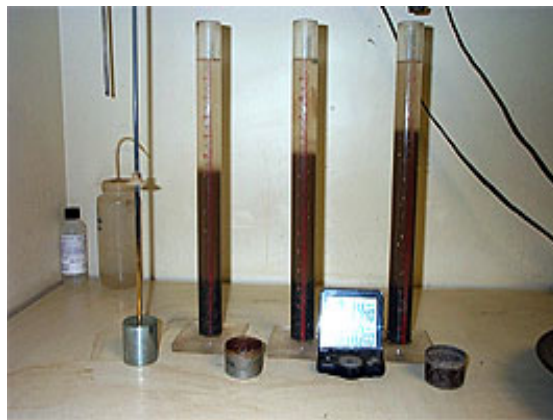
Figure 3.17: Sand Equivalency test tubes with Black Beauty and Silica Sand
