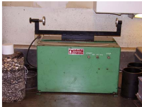
Figure 3.18: Mechanical Shaker used for Sand Equivalency Test
