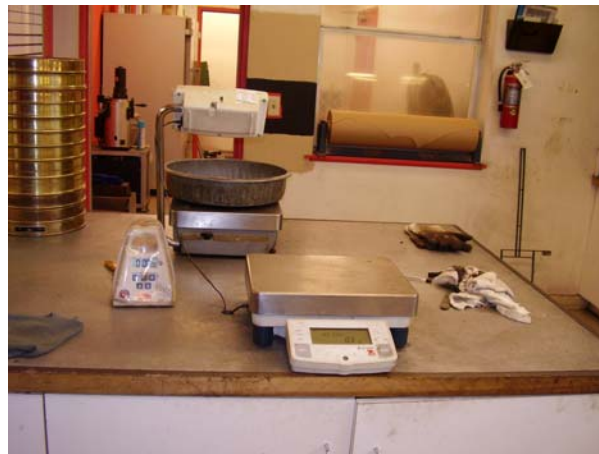
Fig 3.23: Hot bath container and electronic scale
