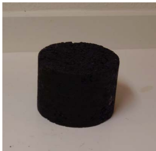
Fig 3.22: Marshal Specimen (4-in diameter and 2.5-inch height)
