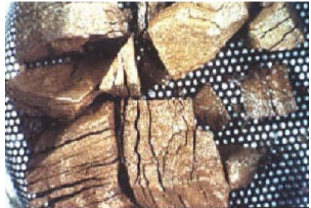
Figure 3.4: Aggregates After a Soundness Test
