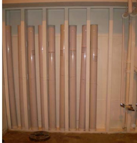
Figure 3.28: PVC with asphalt specimens submerged
