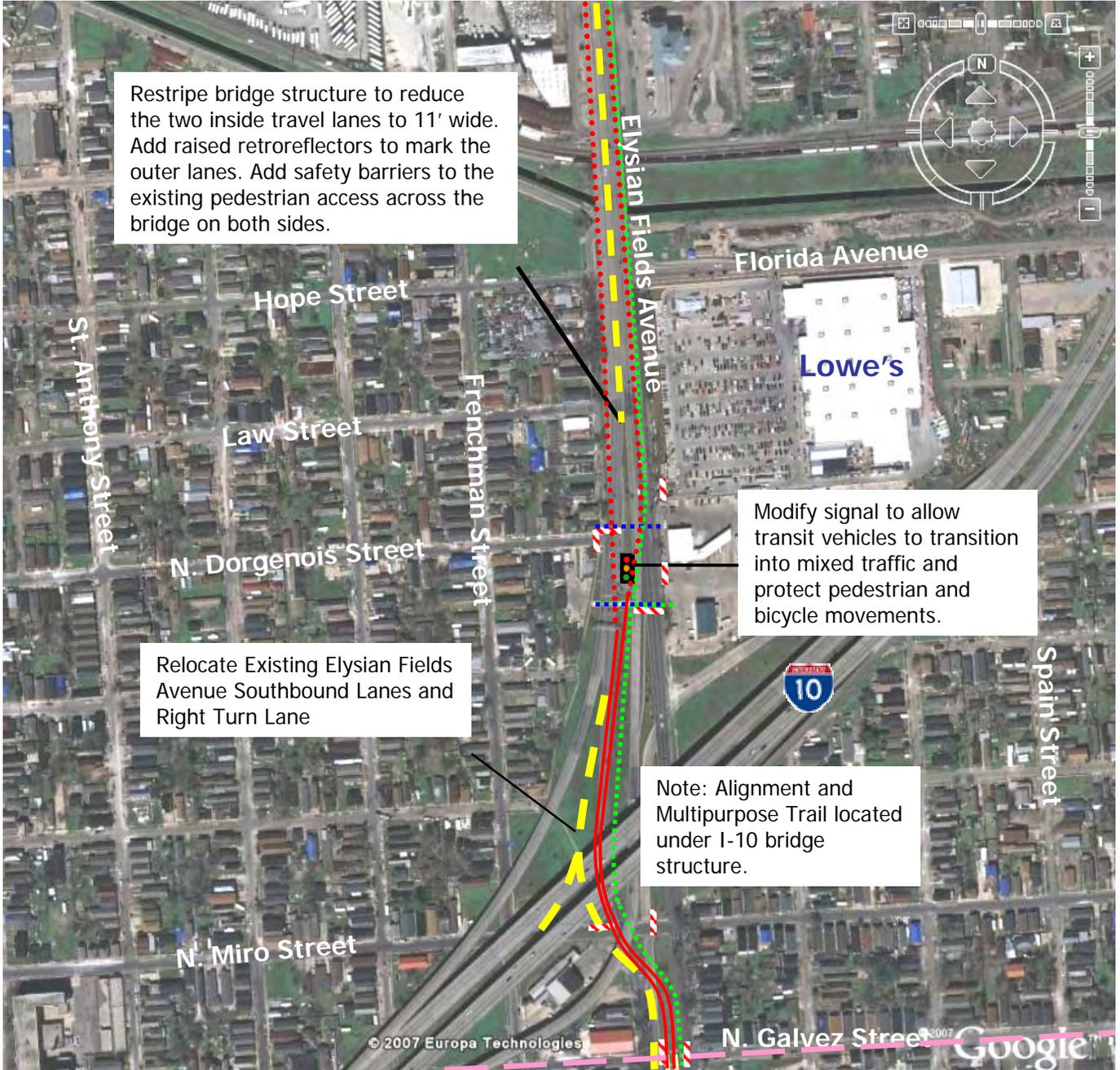
Restripe bridge structure to reduce the two inside travel lanes to 11' wide. Add raised retroreflectors to mark the outer lanes. Add safety barriers to the existing pedestrian access across the bridge on both sides.
