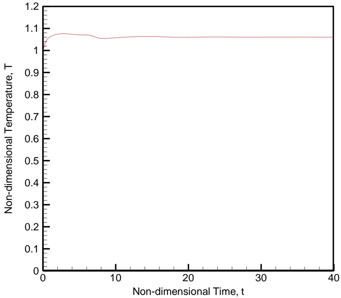
Figure 61- Non-dimensional Temperature Histogram for  $Ra = 10^5$  at  $\bar{x} = 0.05$  and  $\bar{y} = 0.5$  ( $41 \times 41$ ,  $\Delta \bar{t} = 5.0E-6$ ) in Second Order Time Accurate Approximation
