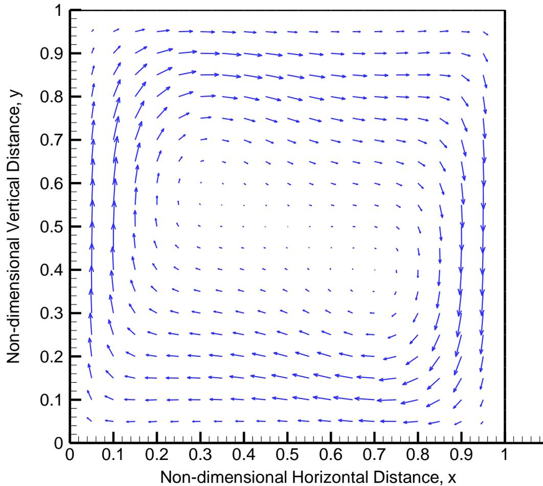
Figure 66- Unsteady State Non-dimensional Velocity Vectors for  $Ra=10^5$  at Non-dimensional Time,  $\bar{t} = 20$  ( $41 \times 41$ ,  $\Delta\bar{t} = 5.0E-6$ ) in Second Order Time Accurate Approximation
