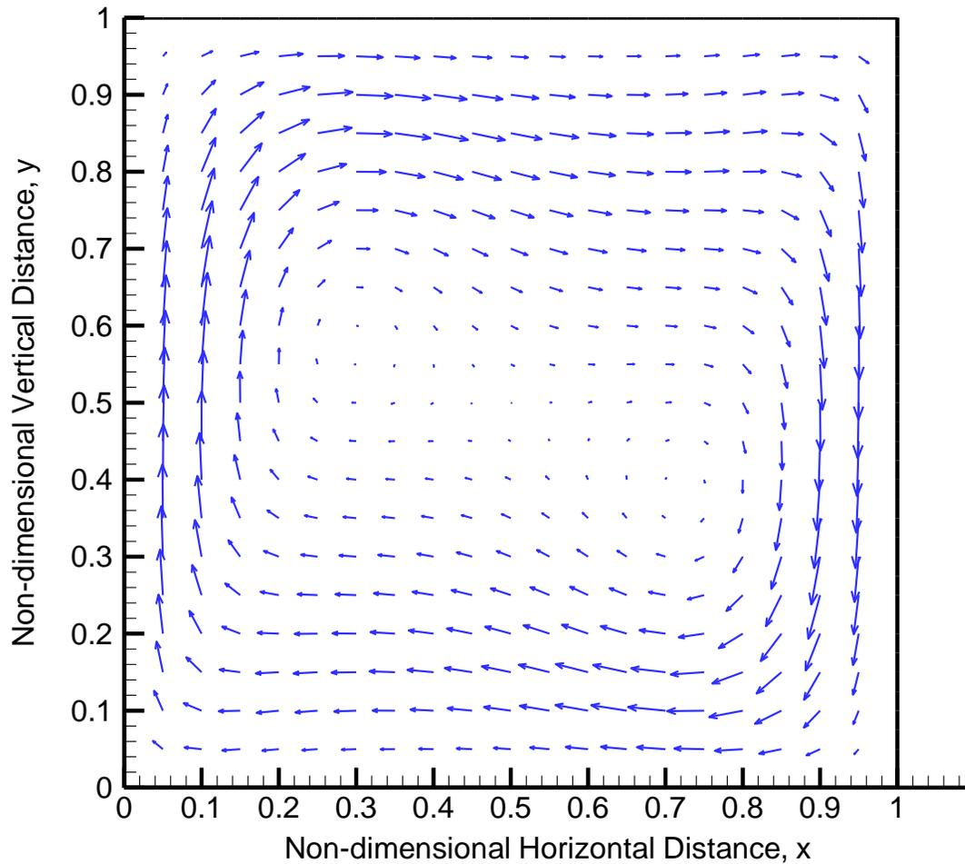
Figure 67- Unsteady State Non-dimensional Velocity Vectors for  $Ra=10^5$  at Non-dimensional Time,  $\bar{t} = 50$  ( $41 \times 41$ ,  $\Delta\bar{t} = 5.0E-6$ ) in Second Order Time Accurate Approximation
