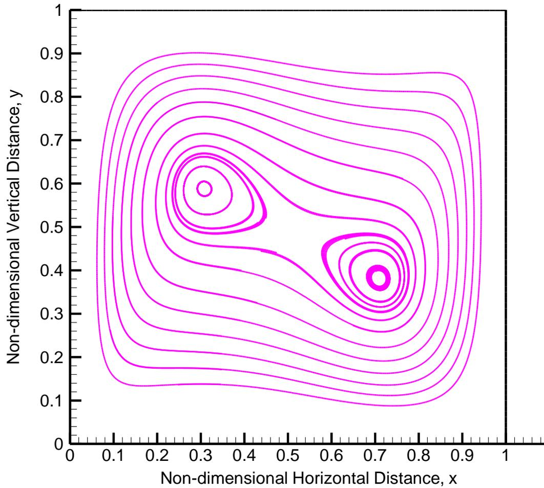
Figure 50- Steady State Non-dimensional Velocity Streamlines for  $Ra=10^5$
