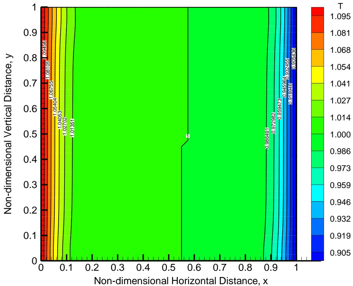
Figure 68- Unsteady State Non-dimensional Temperature Contours for  $Ra=10^5$  at Non-dimensional Time,  $\bar{t} = 1$  ( $41 \times 41$ ,  $\Delta\bar{t} = 5.0E-6$ ) in Second Order Time Accurate Approximation
