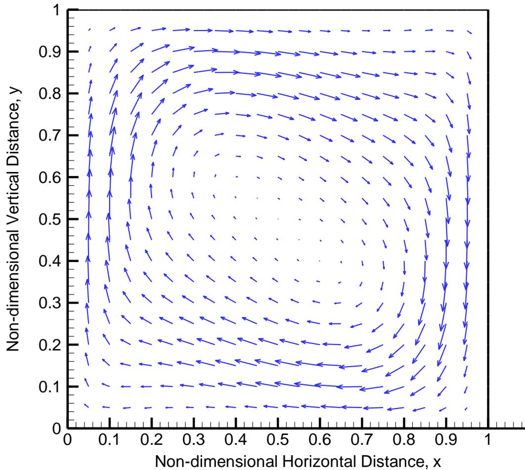
Figure 64- Unsteady State Non-dimensional Velocity Vectors for  $Ra=10^5$  at Non-dimensional Time,  $\bar{t} = 10$  ( $41 \times 41$ ,  $\Delta\bar{t} = 5.0E-6$ ) in Second Order Time Accurate Approximation
