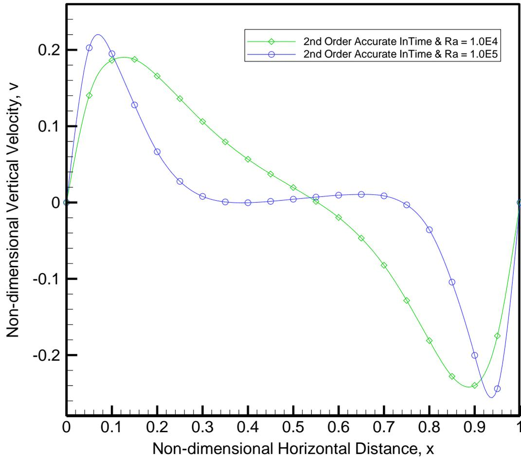
Figure 59- Comparison of Steady State Vertical Velocity Distribution along the Horizontal Centerline of the Enclosure between  $Ra= 10^4$  and  $Ra= 10^5$  in Second Order Time Accurate Approximation
