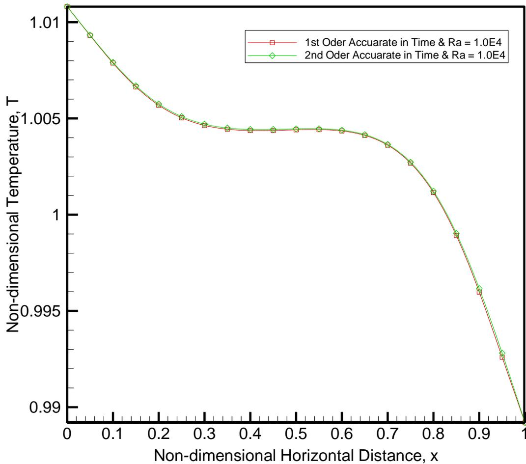
Figure 57- Comparison of Steady State Temperature Distribution along the Horizontal Centerline of the Enclosure between First Order and Second Order Time Accuarate Approximation for Ra=  $10^4$
