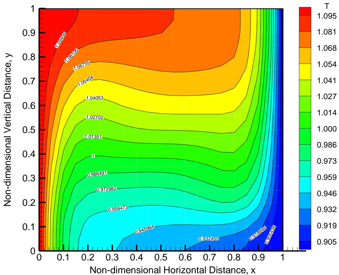
Figure 42- Steady State Non-dimensional Temperature Contours for  $Ra=10^5$
