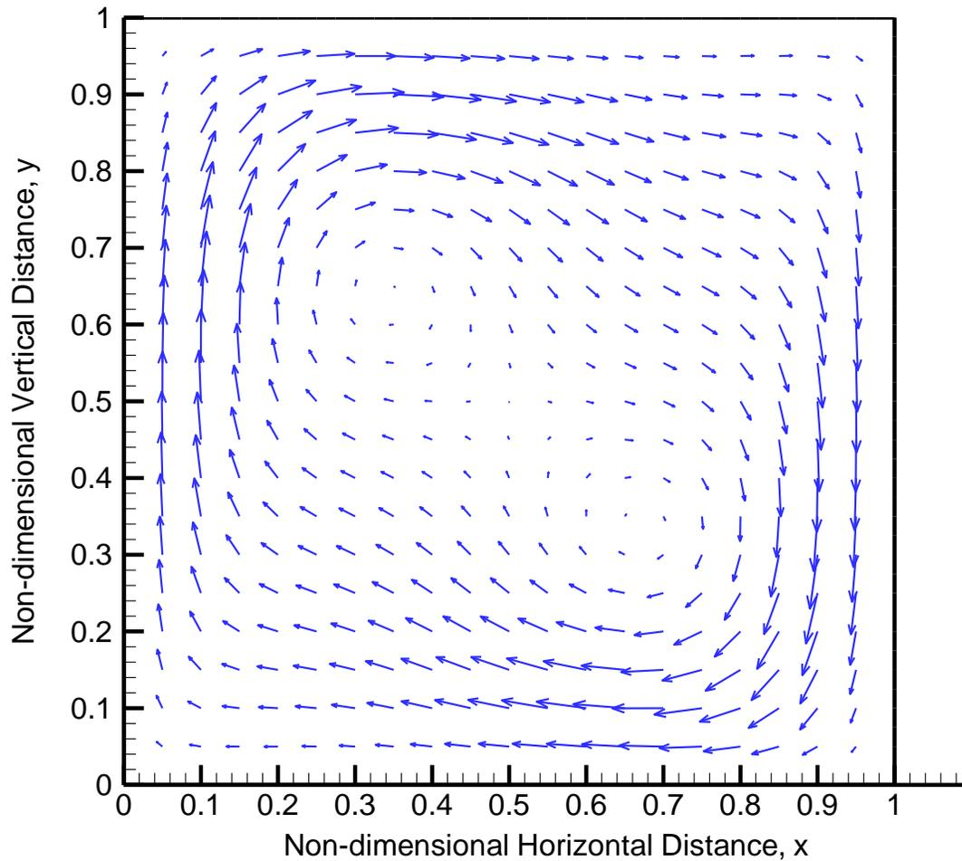
Figure 63- Unsteady State Non-dimensional Velocity Vectors for  $Ra=10^5$  at Non-dimensional Time,  $\bar{t} = 5$  ( $41 \times 41$ ,  $\Delta\bar{t} = 5.0E-6$ ) in Second Order Time Accurate Approximation
