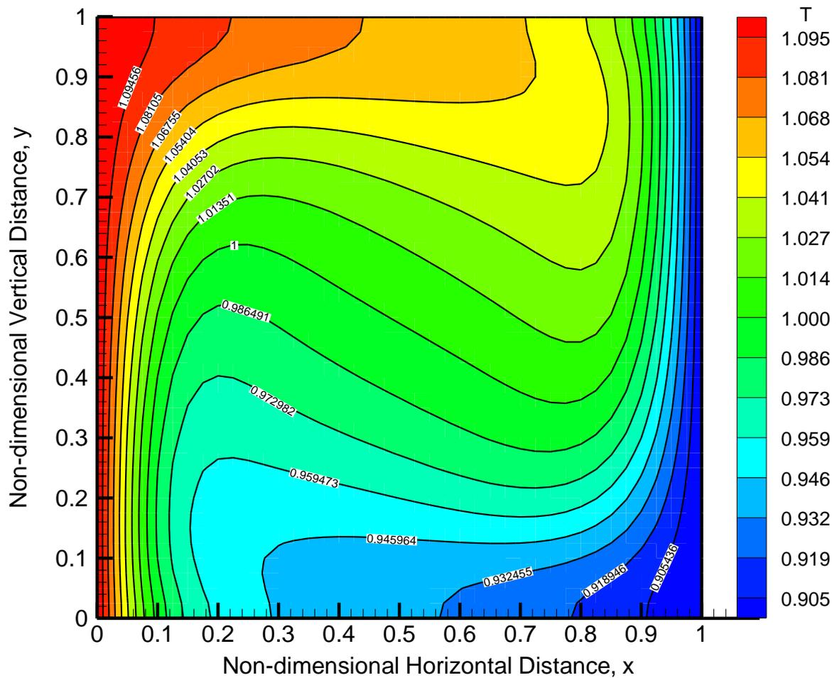
Figure 70- Unsteady State Non-dimensional Temperature Contours for  $Ra=10^5$  at Non-dimensional Time,  $\bar{t} = 10$  ( $41 \times 41$ ,  $\Delta\bar{t} = 5.0E-6$ ) in Second Order Time Accurate Approximation
