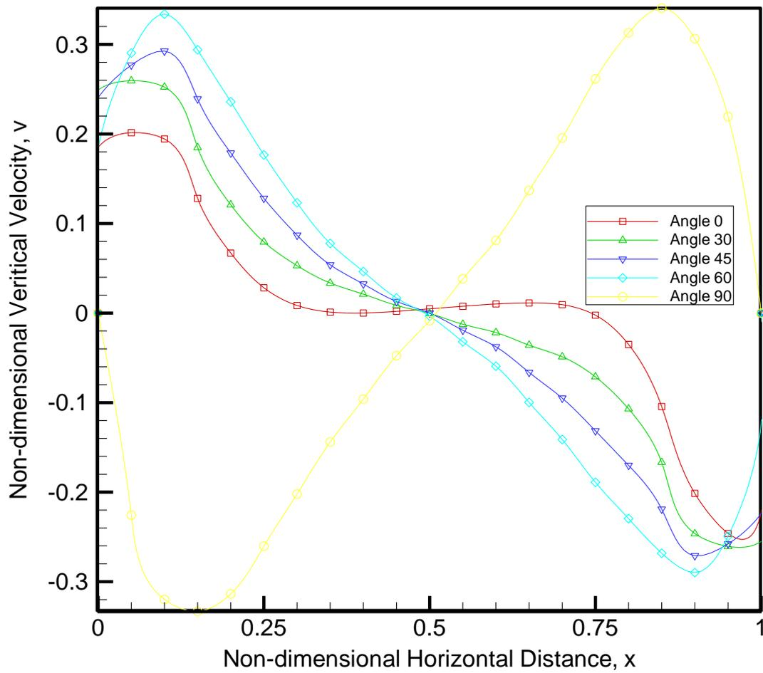
Figure 37- Steady State Non-dimensional Vertical Velocity Distributions along the Horizontal Centerline of the Inclined Enclosure for Constant Fluid Properties at  $Ra= 10^5$
