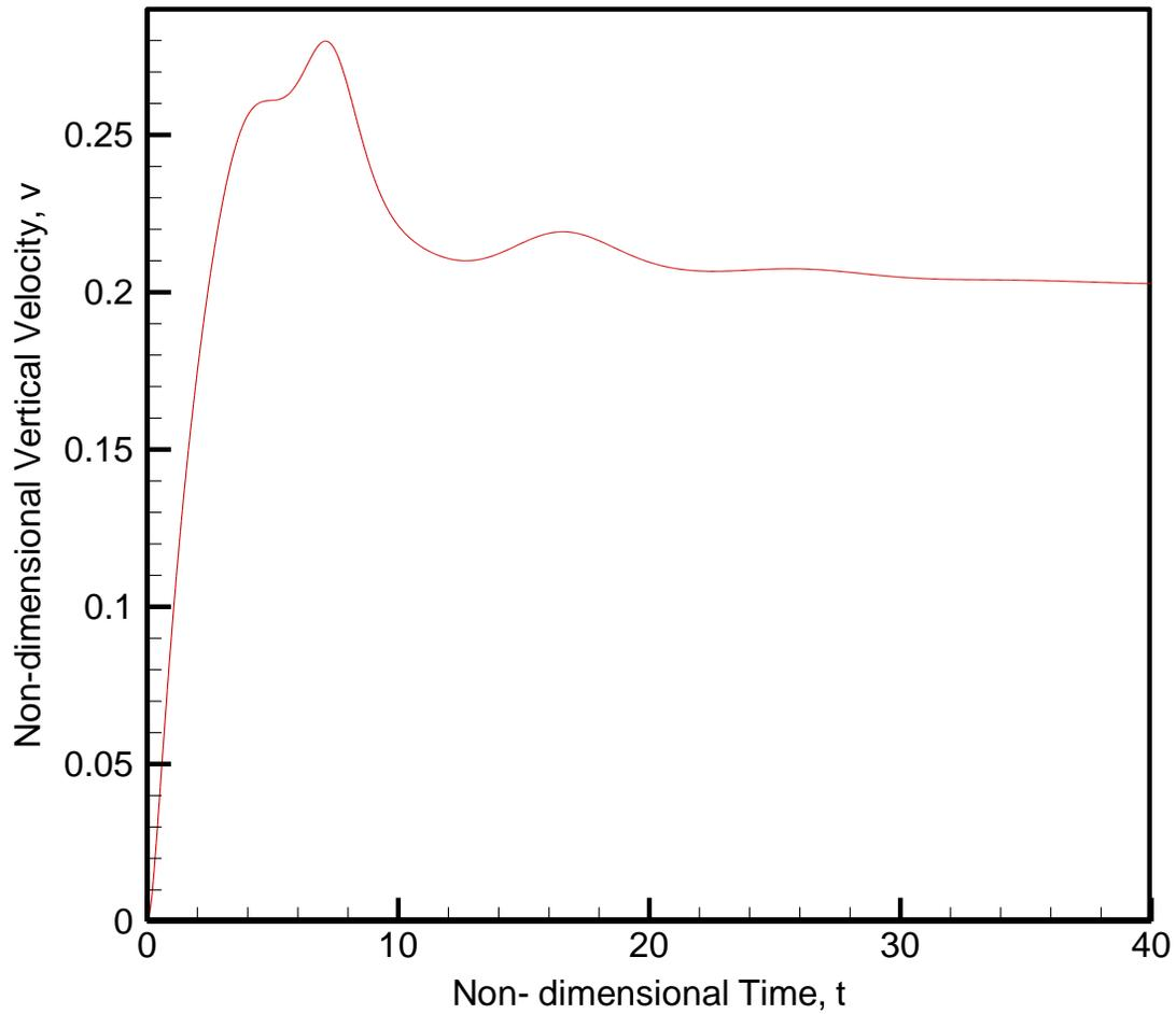
Figure 41- Non-dimensional Vertical Velocity Histogram for  $Ra=10^5$  at  $\bar{X}=0.2$  and  $\bar{Y}=0.5$  ( $21 \times 21$ ,  $\Delta \bar{t} = 1.0E-5$ ) in Second Order Time Accurate Approximation
