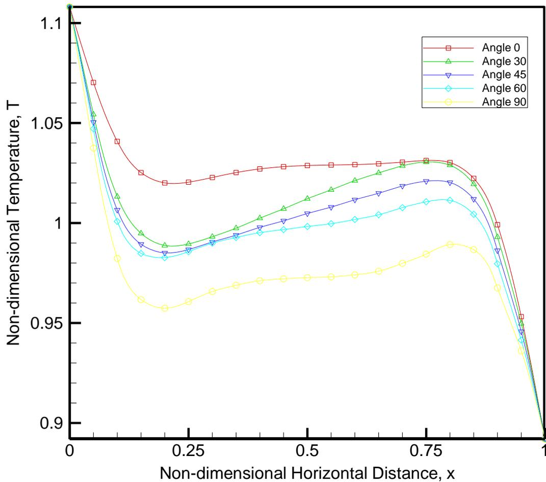
Figure 38- Steady State Non-dimensional Temperature Distributions along the Horizontal Centerline of the Inclined Enclosure for Constant Fluid Properties at  $Ra= 10^5$
