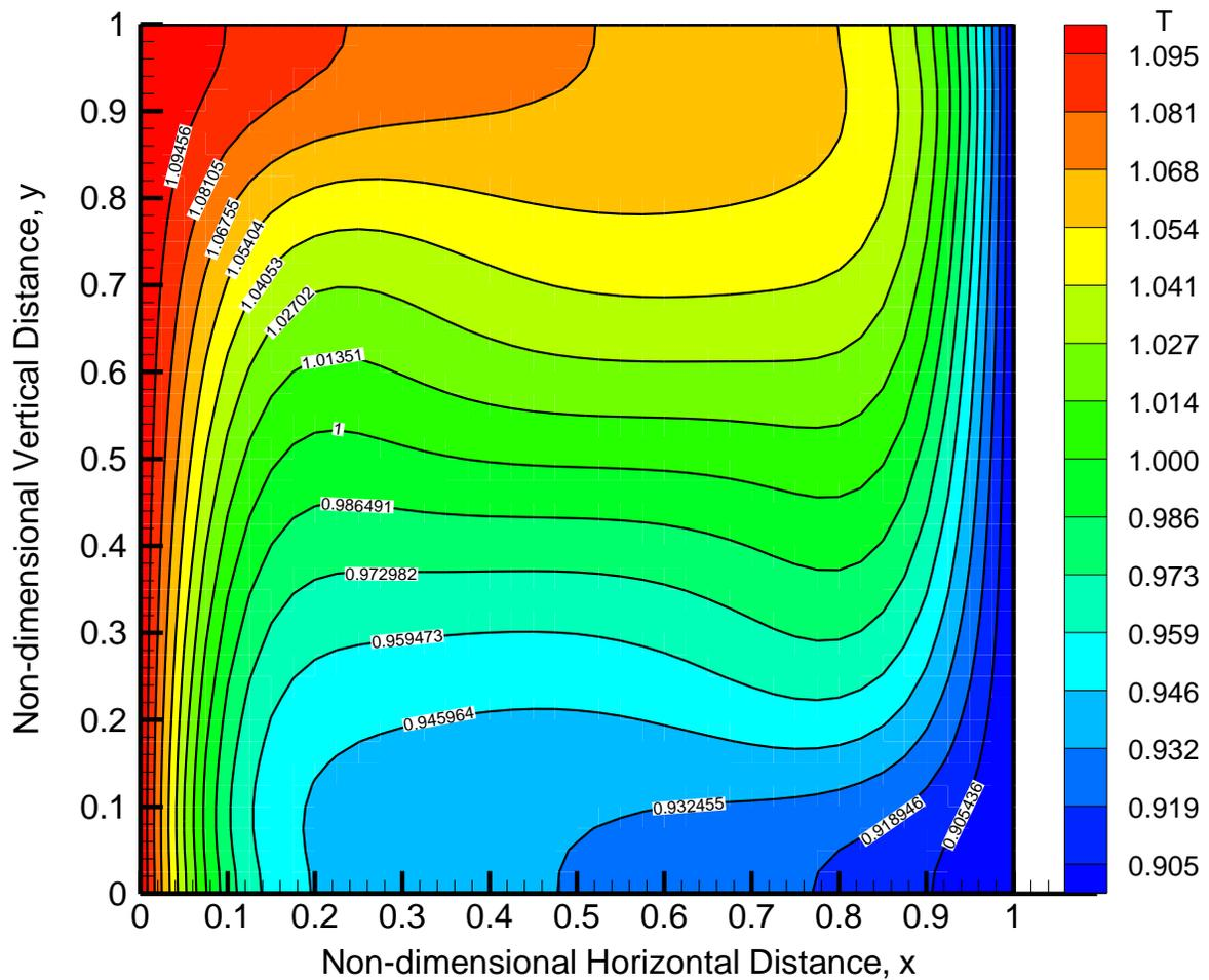
Figure 73- Unsteady State Non-dimensional Temperature Contours for  $Ra=10^5$  at Non-dimensional Time,  $\bar{t} = 50$  ( $41 \times 41$ ,  $\Delta\bar{t} = 5.0E-6$ ) in Second Order Time Accurate Approximation
