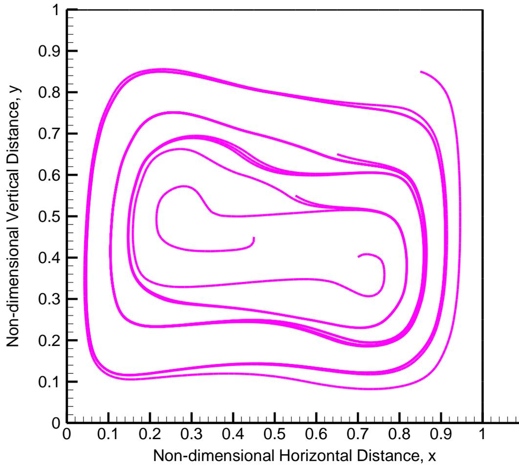
Figure 44- Steady State Non-dimensional Velocity Streamlines for  $Ra=10^5$
