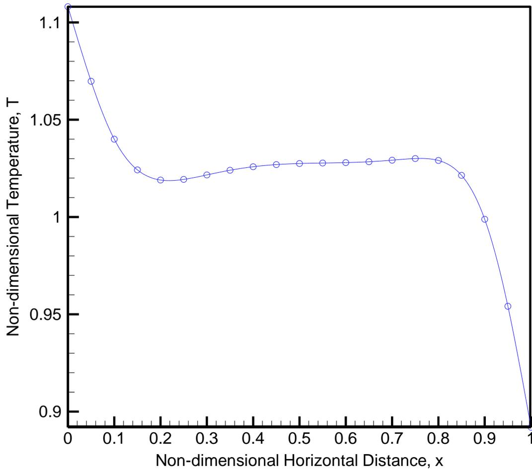
Figure 47- Steady State Non-dimensional Temperature Distribution along the Horizontal Centerline of the Enclosure for  $Ra=10^5$  ( $21 \times 21$ ,  $\Delta \bar{t} = 1.0E-5$ ) in Second Order Time Accurate Approximation
