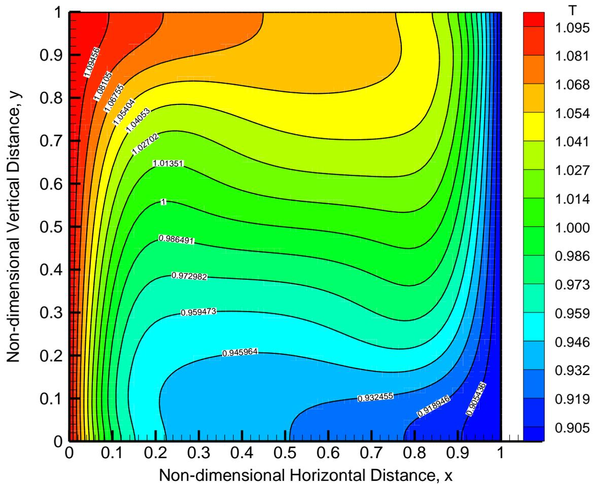
Figure 51- Steady State Non-dimensional Temperature Contours for  $Ra=10^5$
