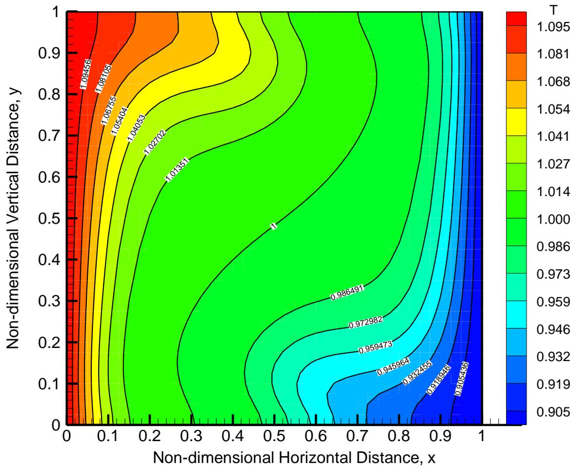
Figure 69- Unsteady State Non-dimensional Temperature Contours for  $Ra=10^5$  at Non-dimensional Time,  $\bar{t} = 5$  ( $41 \times 41$ ,  $\Delta\bar{t} = 5.0E-6$ ) in Second Order Time Accurate Approximation
