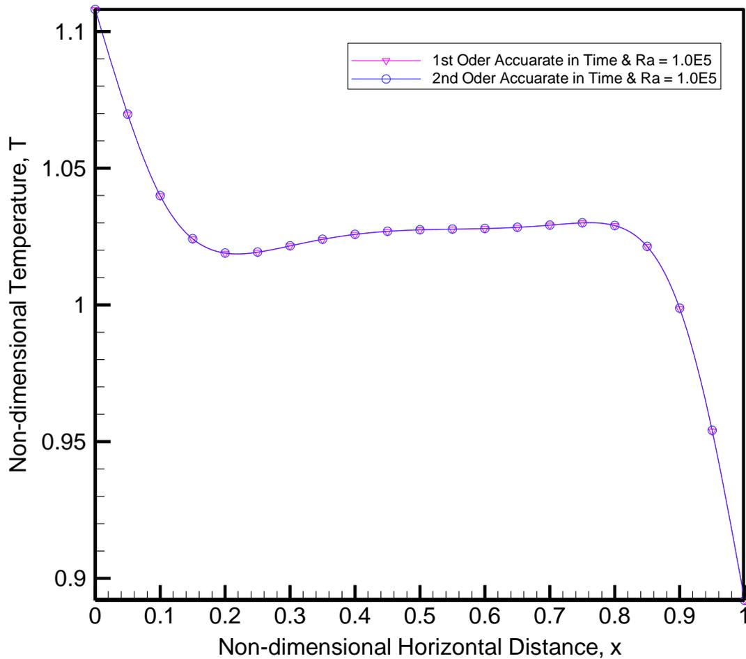
Figure 54- Comparison of Steady State Temperature Distribution along the Horizontal Centerline of the Enclosure between First Order and Second Order Time Accuarate Approximation for Ra=  $10^5$
