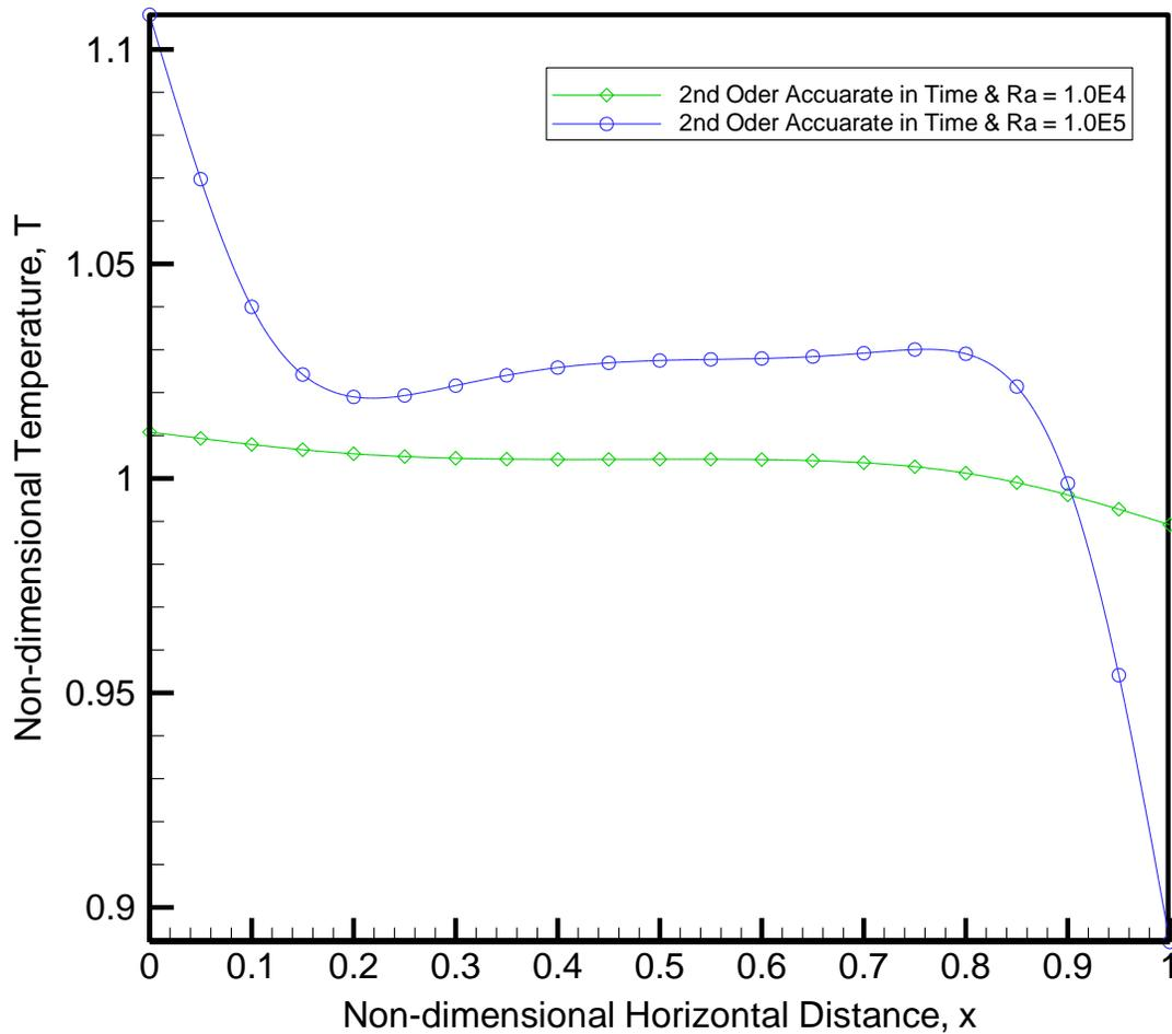
Figure 60- Comparison of Steady State Temperature Distribution along the Horizontal Centerline of the Enclosure between  $Ra= 10^4$  and  $Ra= 10^5$  in Second Order Time Accuarate Approximation
