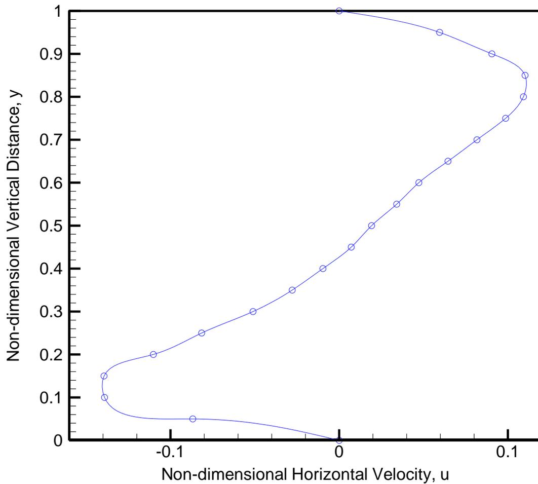
Figure 45- Steady State Non-dimensional Horizontal Velocity Distribution along the Vertical Centerline of the Enclosure for  $Ra=10^5$  ( $21 \times 21$ ,  $\Delta\bar{t} = 1.0E-5$ ) in Second Order Time Accurate Approximation
