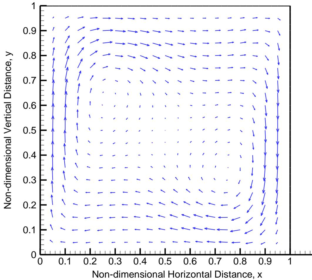
Figure 65- Unsteady State Non-dimensional Velocity Vectors for  $Ra=10^5$  at Non-dimensional Time,  $\bar{t} = 15$  ( $41 \times 41$ ,  $\Delta\bar{t} = 5.0E-6$ ) in Second Order Time Accurate Approximation
