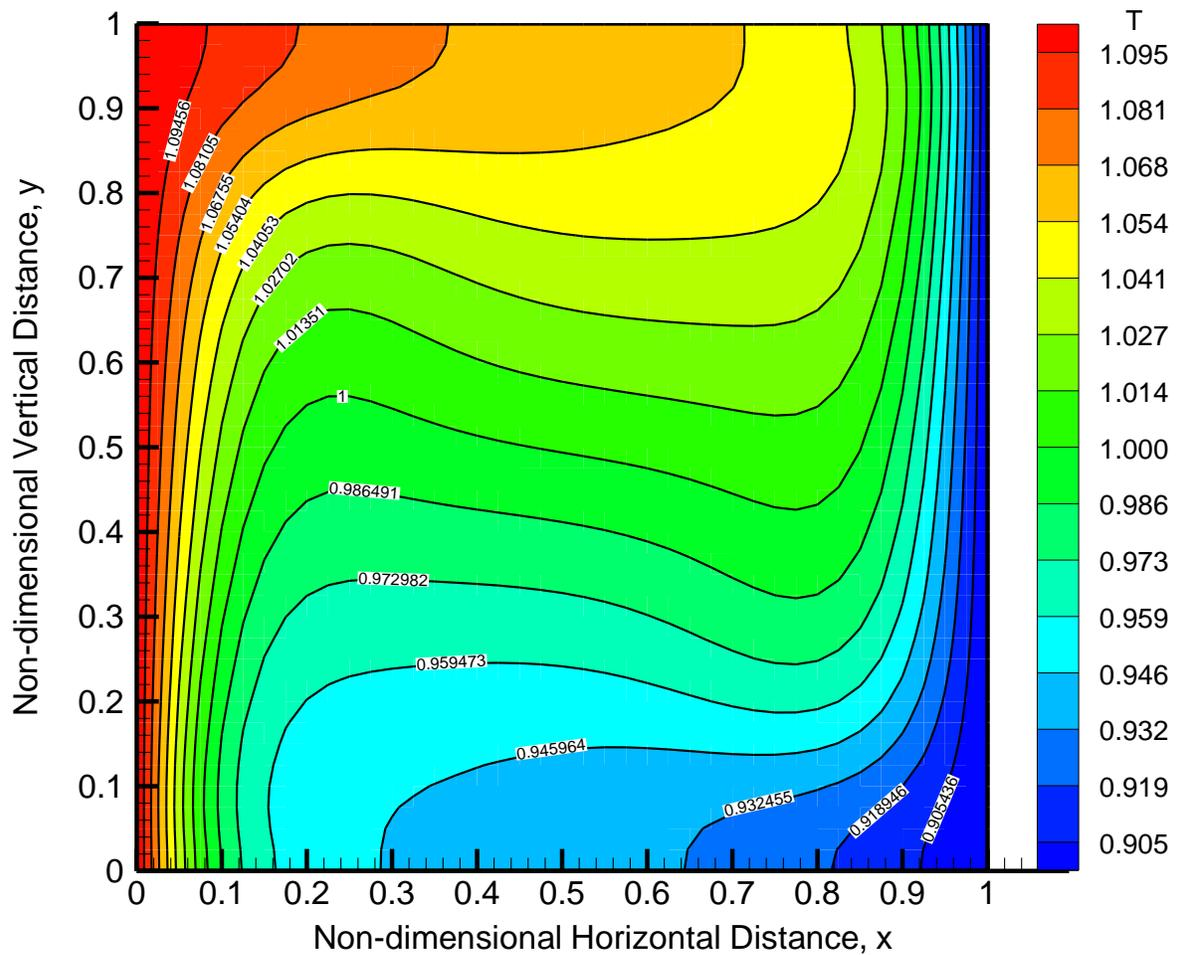
Figure 71- Unsteady State Non-dimensional Temperature Contours for  $Ra=10^5$  at Non-dimensional Time,  $\bar{t} = 15$  ( $41 \times 41$ ,  $\Delta\bar{t} = 5.0E-6$ ) in Second Order Time Accurate Approximation
