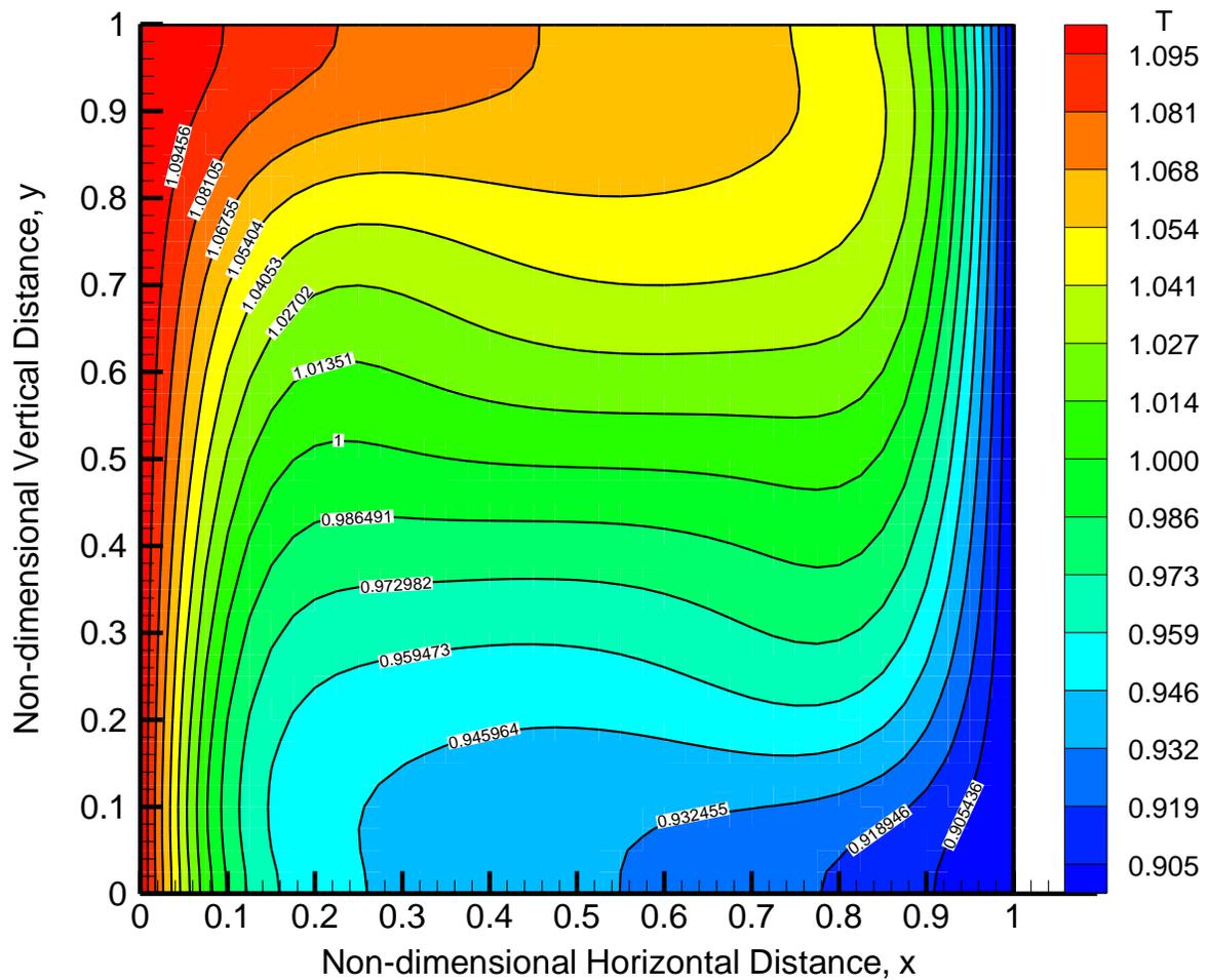
Figure 72- Unsteady State Non-dimensional Temperature Contours for  $Ra=10^5$  at Non-dimensional Time,  $\bar{t} = 20$  ( $41 \times 41$ ,  $\Delta\bar{t} = 5.0E-6$ ) in Second Order Time Accurate Approximation
