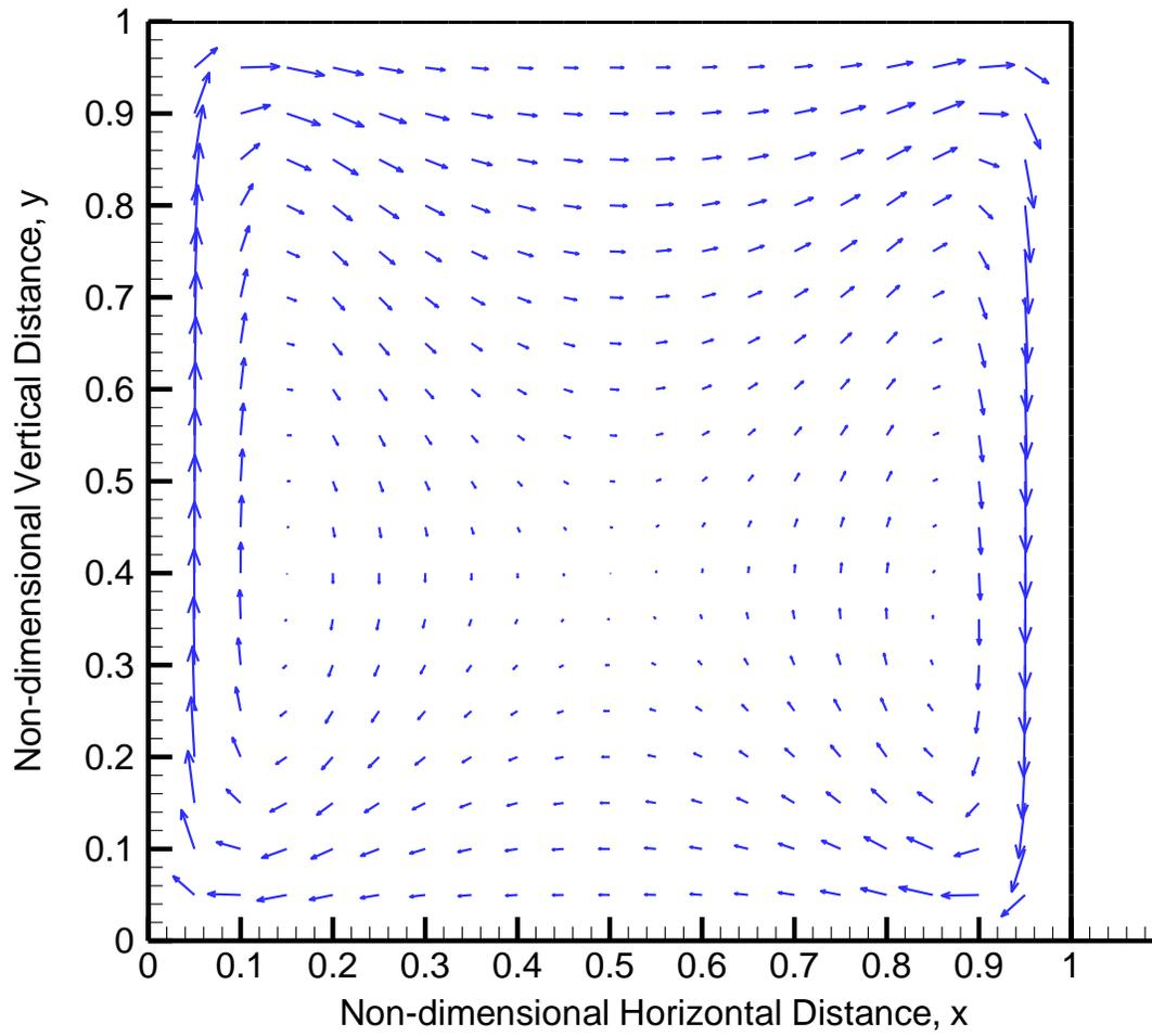
Figure 62- Unsteady State Non-dimensional Velocity Vectors for  $Ra=10^5$  at Non-dimensional Time,  $\bar{t} = 1$  ( $41 \times 41$ ,  $\Delta\bar{t} = 5.0E-6$ ) in Second Order Time Accurate Approximation
