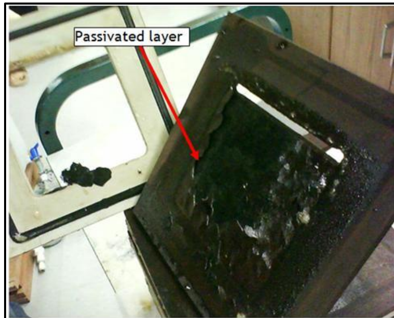
Figure 2.4. Iron electrode with a passivated layer after EC process
