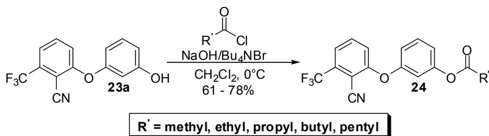
The diaryl ether phenol **23a** undergoes phase transfer catalysis with the appropriate acid halide, 45% NaOH and tetrabutylammonium bromide at 0 °C to afford the desired diaryl ether ester analogue **24**.
