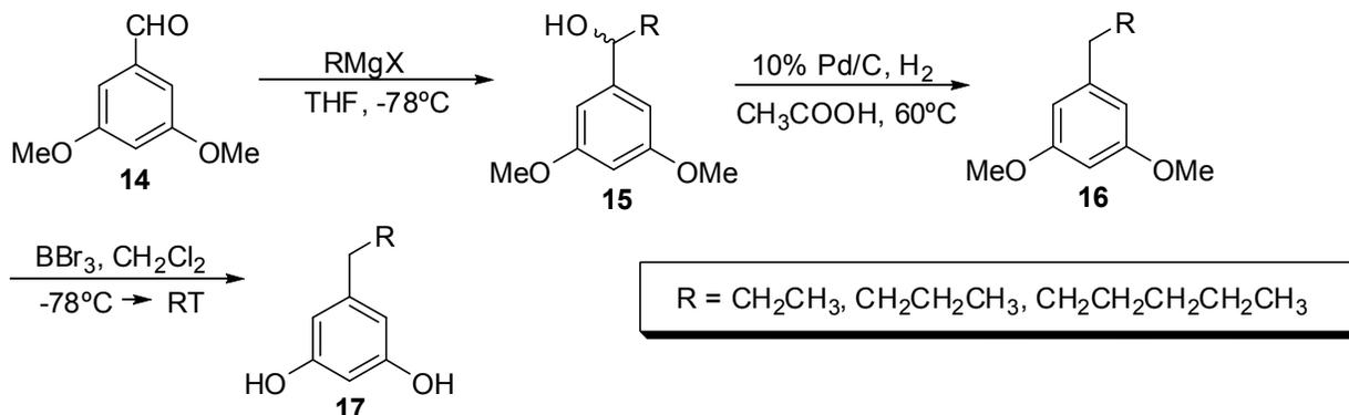
The alcohol **15** was then deoxygenated under catalytic hydrogenolysis using 10%Pd/C and a hydrogen balloon in glacial acetic acid at 60 °C to furnish the resorcinol dimethyl ether **16**. The dimethyl ether groups of **16** were deprotected with BBr<sub>3</sub> at -78 °C to give the desired 5-alkylbenzene-1,3-diol **17**. This procedure was employed to synthesize the propyl, butyl, and hexyl benzene-1,3-diols in 99%, 88%, and 99% yield, respectively.
