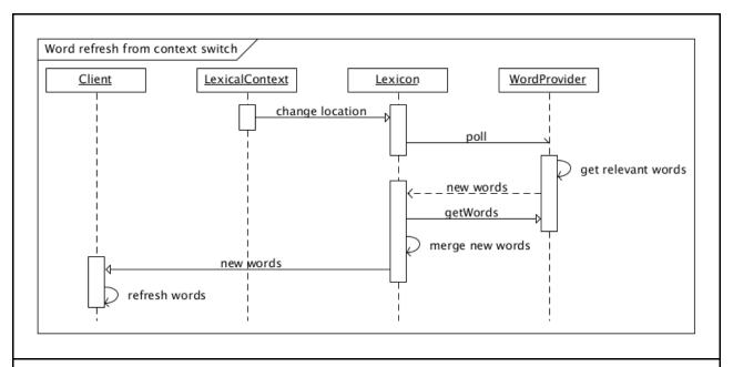
Figure 2. Sequence Diagram showing the interaction between the Lexicon and WordProviders triggered by events from the client user interface.
