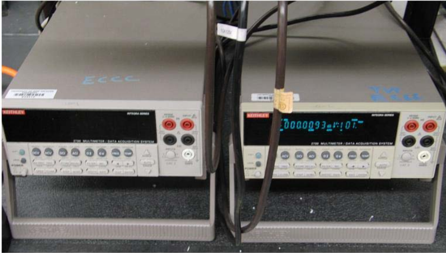
Figure 2.25 Keithley model 2700-multimeter/data acquisition systems with 48 channels of differential ports.
