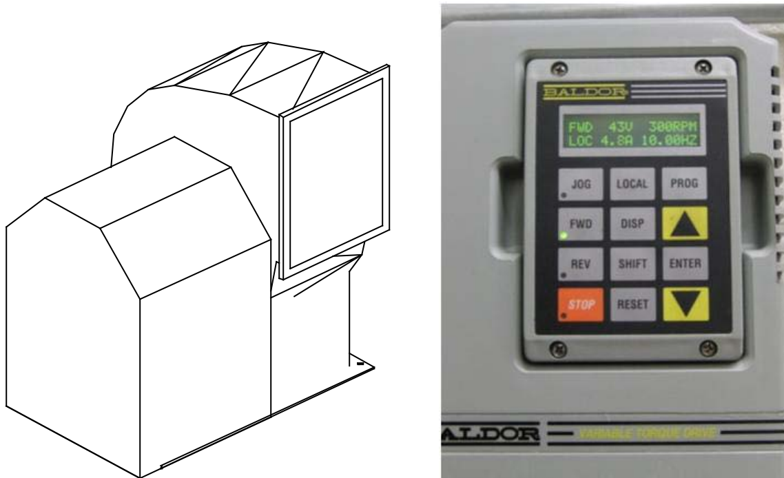
Figure 2.3 Fan, motor, inlet vane control and variable speed drive
