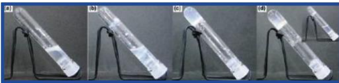
Figure 1.18 Gel experimental results depicted in which mixtures of of the four previously mentioned chloroalkanes, (a) \text{CH}_2\text{Cl}_2 , (b) \text{CHCl}_3 , (c) 1,1,2-trichloroethane, and (d) 1,1,2,2-tetrachloroethane and tris-urea gel compound 17 . Reprinted with permission from Yamanaka, M.; Fujii, H.; J. Org. Chem. , 2009 , 74 , 5390–5394. Copyright 2009 American Chemical Society
