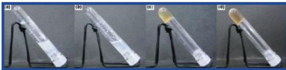
Figure 1.19 Photographs acquired by Fujii et al of \text{CuBr}_2 doped gels of 17 along with the standard chloroalkanes (a) \text{CH}_2\text{Cl}_2 , (b) \text{CHCl}_3 , (c) 1,1,2-trichloroethane, and (d) 1,1,2,2-tetrachloroethane. Reprinted with permission from Yamanaka, M.; Fujii, H.; J. Org. Chem. , 2009 , 74 , 5390–5394. Copyright 2009 American Chemical Society
