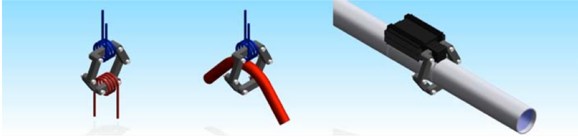
Figure 5. The HydroFlow (right) unit works as a transformer (left). (Rodriguez, 2012)
