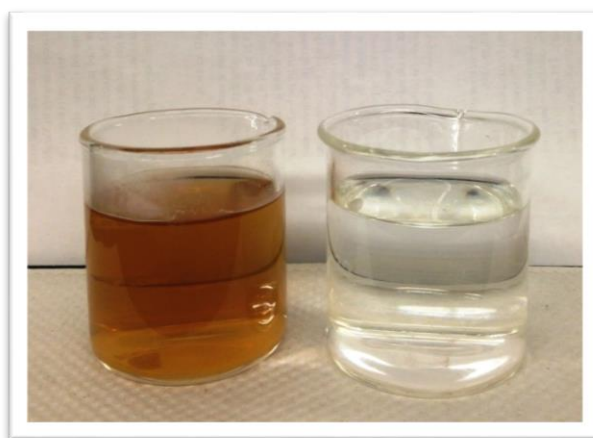
Figure 4.2. From left to right: Effluent of 24-h photocatalytic treatment (without aeration); effluent of 24-h photocatalytic treatment (with aeration).
