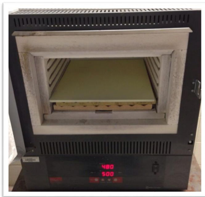
Figure 3.2. Titanium plate coated by spray pyrolysis.
