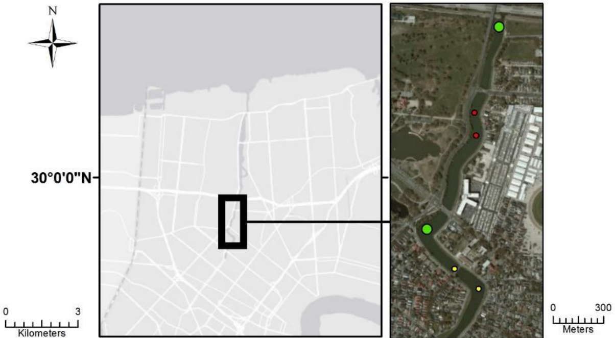
Figure 2.2. Map generated using ArcMap 10 showing mooring locations for the range test. Distances of 250, 400, 550, and 675 m were tested. Yellow transmitters were associated with receiver at site CAB (southern site) and red indicates transmitters associated with the receiver at I610 (northern site).
