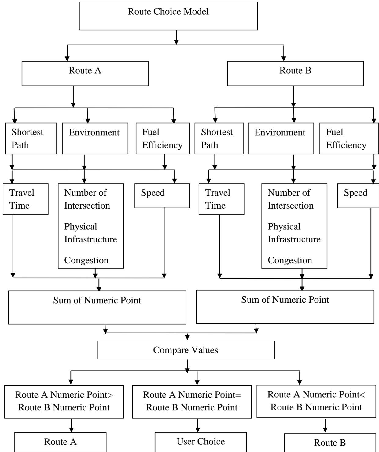
Figure 3.2: Flow chart of model used for case studies
