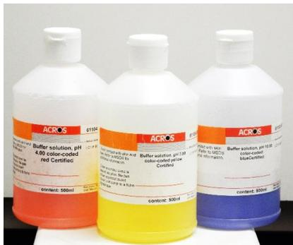
Figure 45. Buffer solutions for pH meter.
