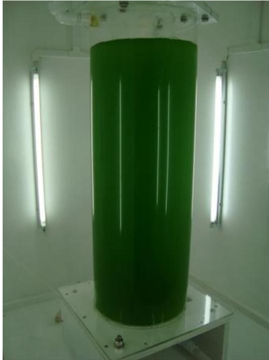
*Figure 7. Photobioreactor internally illuminated. SOURCE: American Society of Mechanical Engineers (ASME).*
