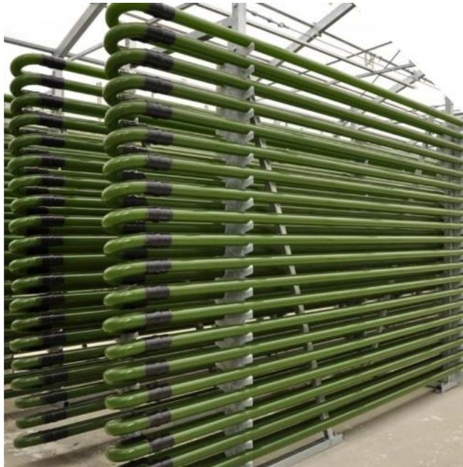
Figure 5. Tubular photobioreactor. SOURCE: [www.bbi-biotech.com](http://www.bbi-biotech.com)
