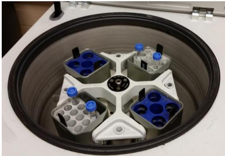
Figure 56. Samples inside the centrifuge.
