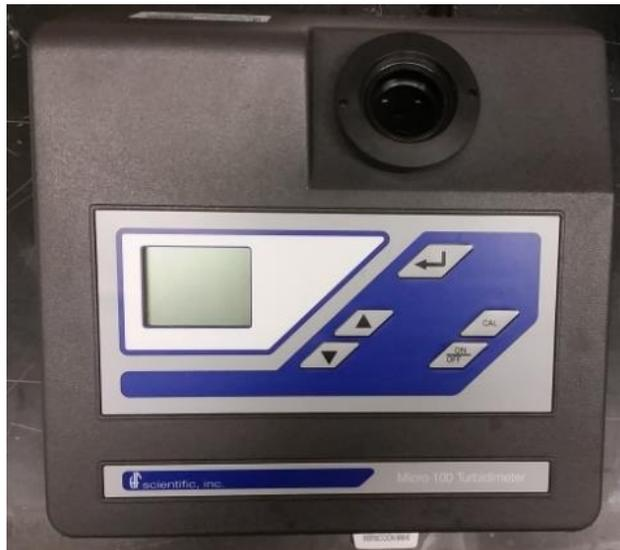
*Figure 52. Turbidimeter.*
