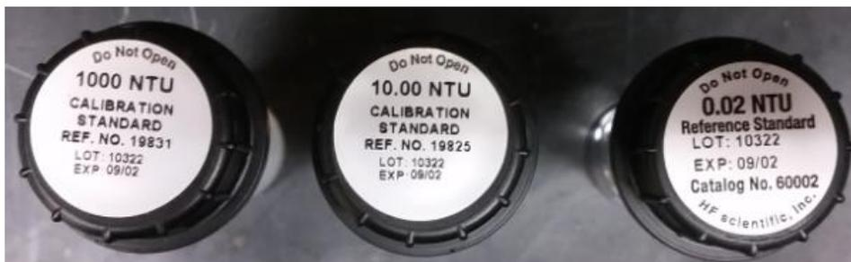
*Figure 53. Turbidimeter calibration set.*
