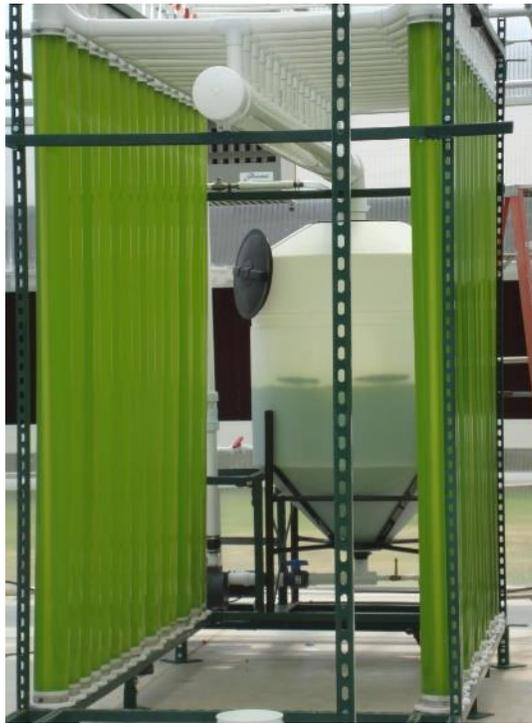
*Figure 6. Vertical photobioreactor. SOURCE: University of Kentucky. Center for Applied Energy Research (CAER). Department of Biosystems & Agricultural Engineering (BAE).*
