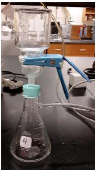
*Figure 54. Filtering Apparatus completely assembled.*
