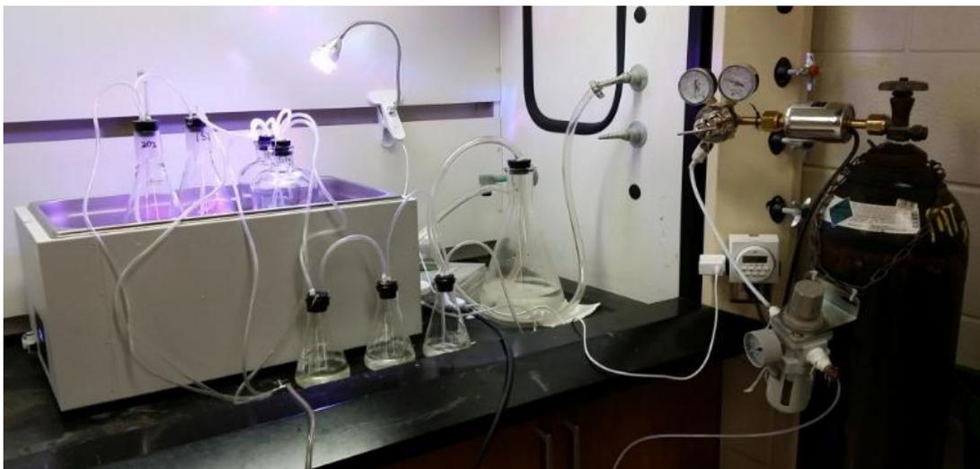
Figure 26. Experiment 1 set up, showing the connections between the flasks, air supply and CO<sub>2</sub> cylinder.
