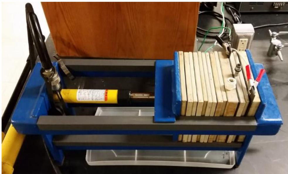
*Figure 21. Electrochemical batch reactor.*
