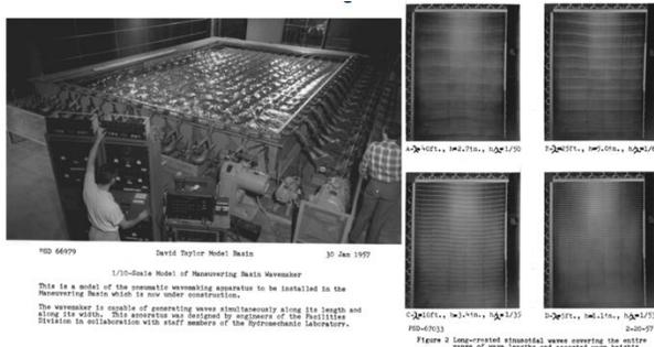
Figure 12. 1/10<sup>th</sup> Scale Model of the MASK Basin.
