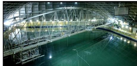
Figure 4. Curved Corner of New EDL 216 Paddle Directional Wavemaker
