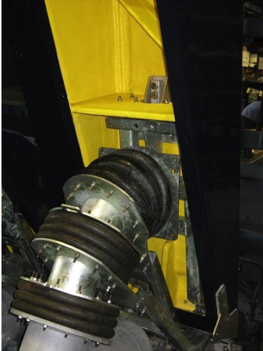
Figure 18. Bellows and Lower Force Transducer
