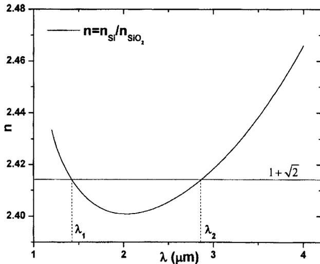
Fig. 3. Relative refractive index of the  $\text{SiO}_2$ -Si interface, Eq. (18), is plotted as a function of wavelength in  $\lambda$   $\mu\text{m}$ . Note that  $n(\lambda) = (1 + \sqrt{2}) = 2.4142$  at two wavelengths  $\lambda_1 = 1.4224$   $\mu\text{m}$  and  $\lambda_2 = 2.8644$   $\mu\text{m}$  (after Ref. 15).
