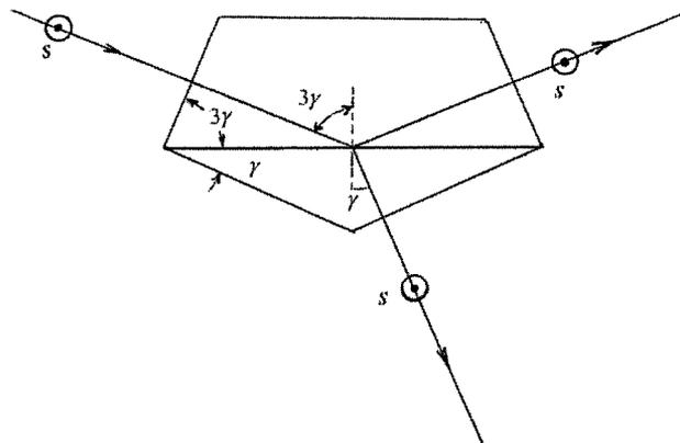
Fig. 2. Biprism BS for  $s$ -polarized light consists of a top prism of  $\text{SiO}_2$ , which is optically contacted to a bottom prism of Si. The angle  $\gamma$  is  $22.5^\circ$  and all other angles are integral multiples of  $\gamma$ . The angle of incidence of  $s$ -polarized light at the  $\text{SiO}_2$ -Si interface is  $67.5^\circ$ .
