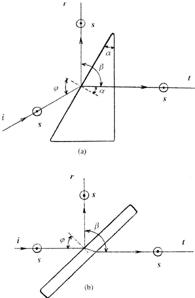
Fig. 1. Cross sections of the (a) prism and (b) slab beam splitters for *s*-polarized light.
