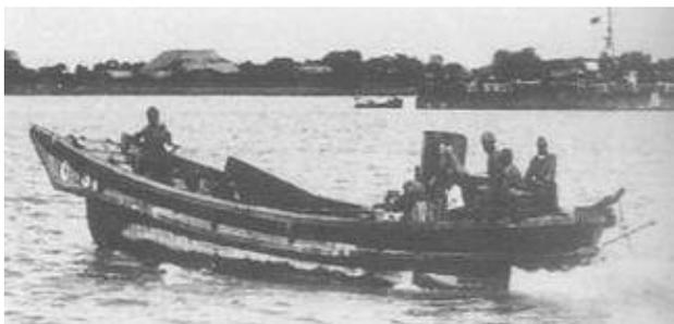
Figure 1. The Daihatsu Class or 14m landing craft used by the Japanese during WWII. (Obtained from World War II Database. Available online. URL: <http://ww2db.com>. Accessed on January 25, 2013).
