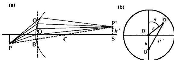
FIG. 3. Configuration for the five Seidel aberrations calculation. (a) Light trace diagram. (b) End-on view of the imaging situation along the axis.  $P$  and  $P'$  are the object and image position, respectively.  $r$  is the aperture stop coordinate vector and  $h'$  is the image plane coordinate vector.
