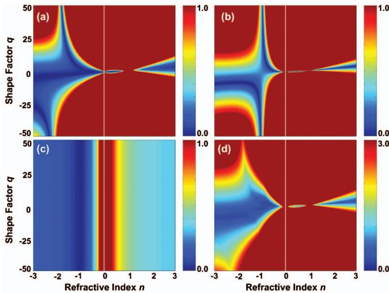
FIG. 4. (Color) Numerical calculated coefficients of the spherical aberration  $C_{040}$  (a), coma  $C_{131}$  (b), curvature  $C_{220}$  (c), and the sum of the three aberrations  $|C_{040}| + |C_{131}| + |C_{220}|$  (d) as a function of the shape factor  $q$  and refractive index  $n$ . The values of the color bars for the spherical aberration, coma, and field curvature range from 0 (navy blue) to 1 (garnet), and the value for the sum spans from 0 to 3.
