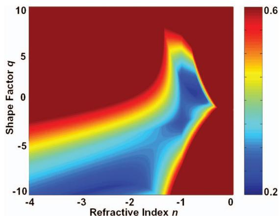
FIG. 5. (Color) Detailed contour map of the area with small values of the sum of the three aberrations  $C_{\text{total}} = |C_{040}| + |C_{131}| + |C_{220}|$ . There are two minimums near the small refractive index area ( $|n| < 2$ ):  $C_{\text{total}} = 0.22$  for  $n = -0.81$  and  $q = 0.83$ ;  $C_{\text{total}} = 0.25$  for  $n = -1$  and  $q = -2.2$ . In order to give the details, the range of the color bar is shrunk to the values from 0.2 to 0.6.
