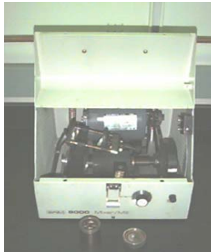
Figure 2.1: Spex Industries 8000 Shaker Mill and Vial
