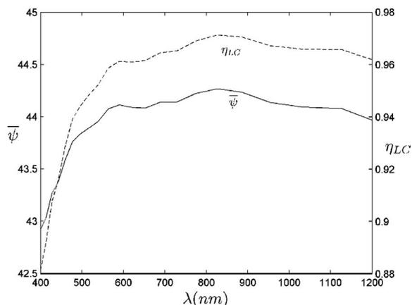
Fig. 6. Linear-to-circular polarization conversion efficiency  $\eta_{LC}$  (dashed curve) and principal azimuth  $\bar{\psi}$  (expanded scale) as functions of wavelength  $\lambda$  for light reflection by a Ag mirror in the visible and near-IR spectral range,  $400 \leq \lambda \leq 1200$  nm. The optical constants of Ag are obtained from [6].
