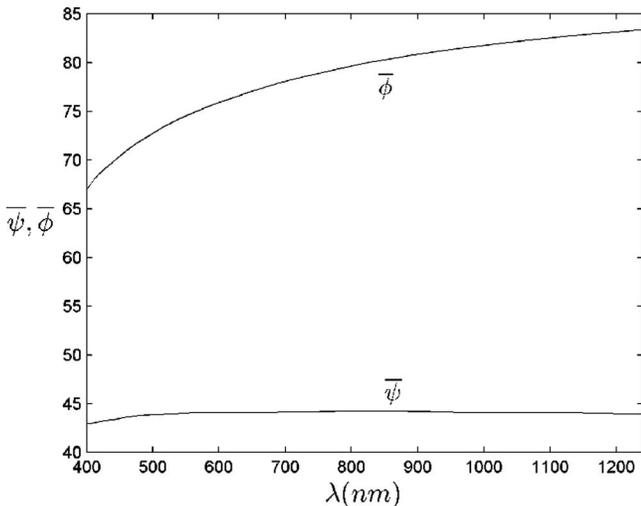
Fig. 5. Principal angle  $\bar{\phi}$  and principal azimuth  $\bar{\psi}$  for light reflection by a Ag mirror in the visible and near-IR spectral range,  $400 \leq \lambda \leq 1200$  nm. The optical constants of Ag are obtained from [6].
