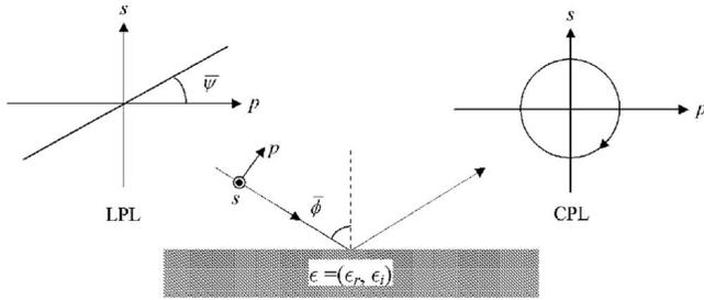
Fig. 1. Incident linearly polarized light (LPL) is reflected circularly polarized (CPL) at the principal angle  $\bar{\phi}$  of a dielectric-conductor interface:  $\bar{\psi}$  is the principal azimuth, and  $p$  and  $s$  represent the orthogonal linear polarization directions parallel and perpendicular to the plane of incidence, respectively.
