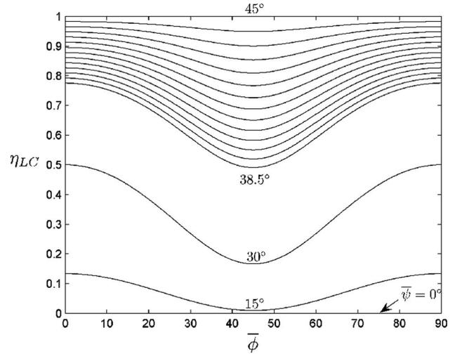
Fig. 2. Efficiency  $\eta_{LC}$  of linear-to-circular polarization conversion as a function of principal angle  $\bar{\phi}$  for constant values of the principal azimuth  $\bar{\psi} = 15^\circ, 30^\circ,$  and  $38.5^\circ$  to  $45^\circ$  in steps of  $0.5^\circ$ .
