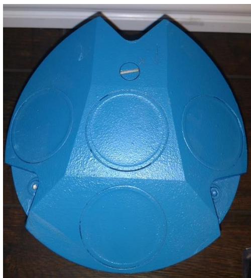
Figure 3. Custom-made ADCP to reduce the effect of the rig legs by facing the transducer sideways. The blue color is antifouling paint that applied before the deployment.
