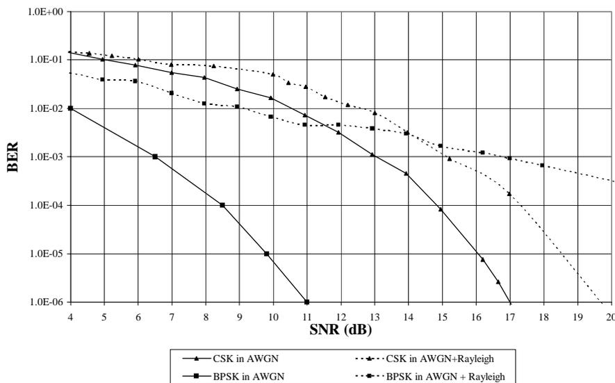
Figure 4: Comparison of CSK to BPSK.
