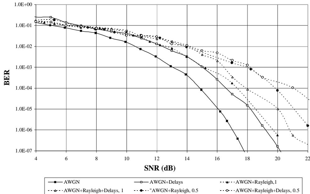
Figure 3: Performance of CSK in terms of probability of error vs SNR for all channels investigated.
