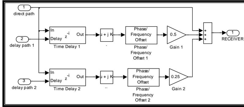
Figure 2: Details of the multipath block.
