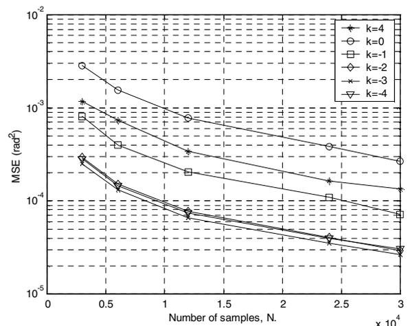
Fig. 7(b). Mean Square Error of Phase Estimates as a function of  $N$  for 128-QAM.  $SNR=31$  dB.
