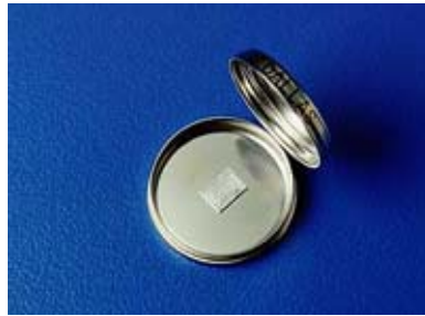
Figure 3.4: Self-powered computer chip in an iButton
