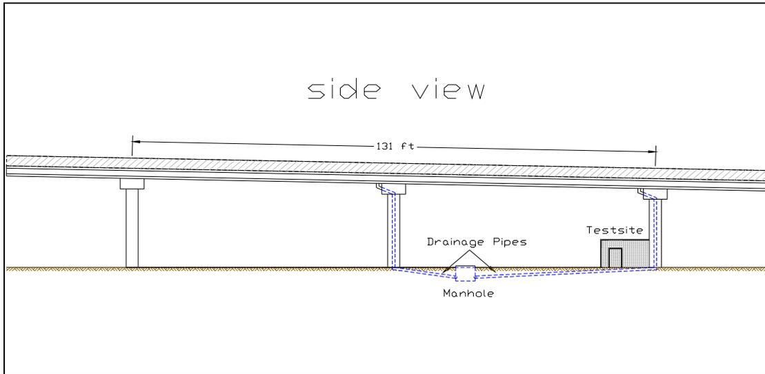
Figure 4: Side View of Section through the Selected I-610 Highway Section at the Experimental Site. [38]
