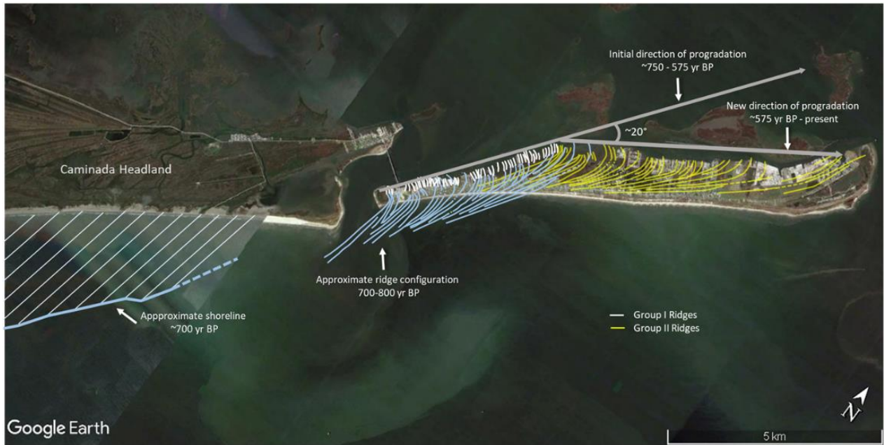
Fig. 11. Schematic of approximate eastern Barataria coastal configuration approximately 0.7 ka. The orientation of Group I ridges and the former position of the Caminada headland shoreline reveal a striking alignment that strongly suggests that erosion rates and change in shoreline configuration of the Caminada headland kept pace with the accretion and directional progradation change of the beach ridges of Grand Isle.
