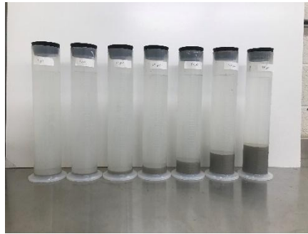
Figure 5.9: 2018-1 mini columns at 2-hour reading (left) and 360-hour reading (right)
