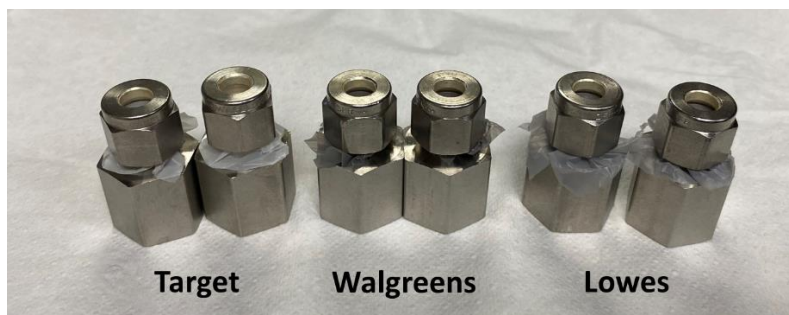
Figure 4.6. Target, Walgreens, Lowes bags secured in 1/4 inch Swagelok fittings.
