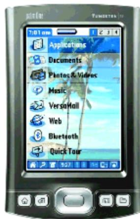
**Figure 1.2 Palm Tungsten T5 with 256MB of internal flash memory.**
