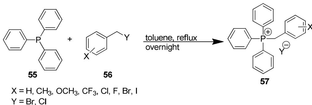
The benzyl halide (3 mL, 21.3 mmol) was added to a dry, 250 mL round-bottom flask containing 1.1 equivalents of triphenylphosphine (5.5 g, 23.4 mmol). The mixture was then dissolved in toluene (70 mL) and refluxed over night. The reaction was cooled to room temperature and filtered. The precipitate (usually a white solid) was washed with diethyl ether (3x50 mL) and dried thoroughly under vacuum before use.
